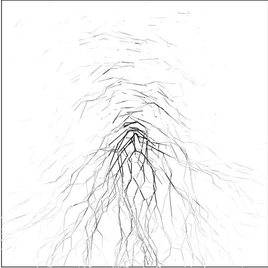
Fig. 6. Picture of a network in the affine stretching dominated regime. The grey-scale is chosen according to the axial force in the segment. No force-chains are present.
