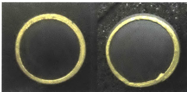
Figure 4-27 membrane sweep side (left) and membrane feed side (right). The membrane was used in the inert gas O 2 permeation experiments and the reactive O 2 permeation experiments in sections 4.2~4.3. Membrane tested for 470hr.
