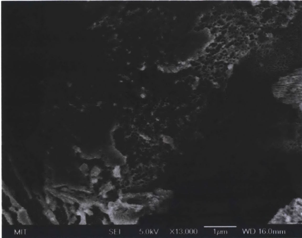
Figure 5-7: SEM image of hierarchical structure at micro scale. HCl was used as an electrolyte for etching process. Nano-structures are observed on micro-structures.
