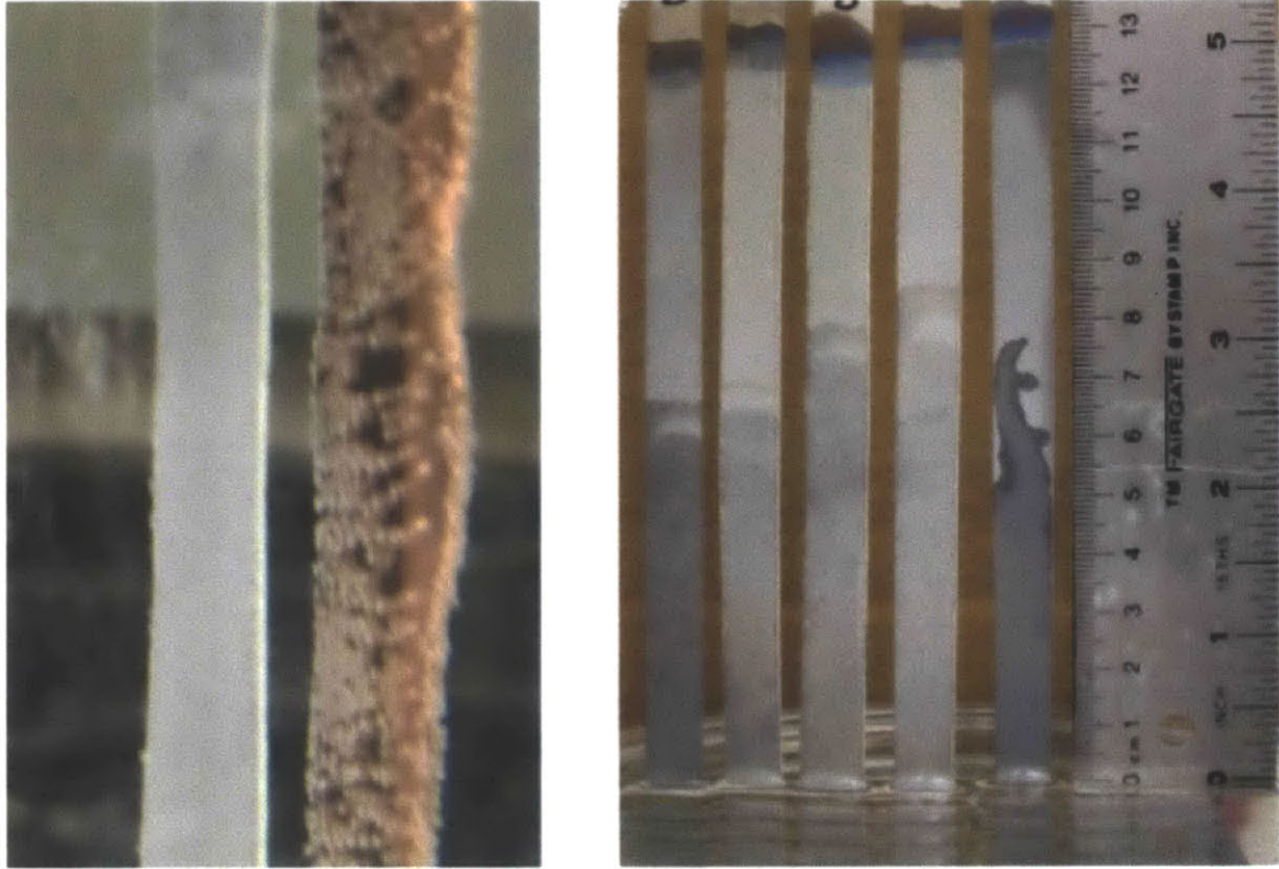
Figure 3-5: Etching Process (left), and capillary rise experiment of etched BDA surface. First sample from the right is etched BDA surface (right).
