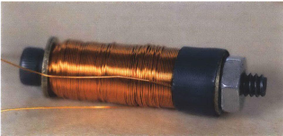
Figure 54: A more typical output from the coil winder.
