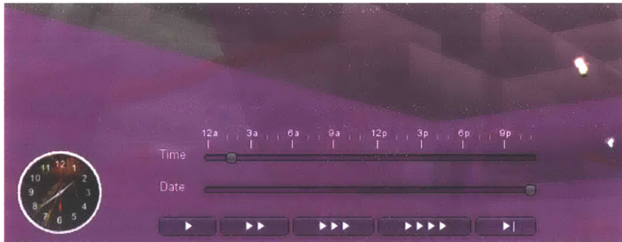
Figure 1-2: The GUI for DoppelLab’s Time Machine functionality. Sliders allow coarse and fine selection of a new time to play back data and sound from; triangle buttons allow selection of playback speed for historical audio (2, 3, and 4 triangles denote speedup factors of 60, 600, and 3600, resp.), the ‘forward’ button returns to real-time data and audio.
