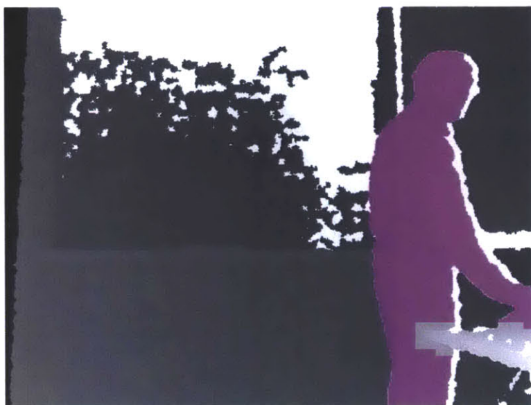
Figure 3-11: Compressed depth stream: darker colors correspond to points that lie further away. Bodies are signified by a hue value.
