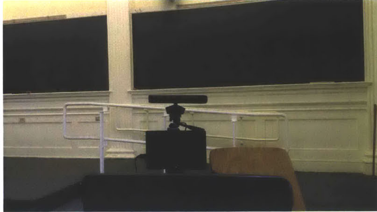
Figure 3-7: Recorder doesn't block board even in unslanted classrooms
