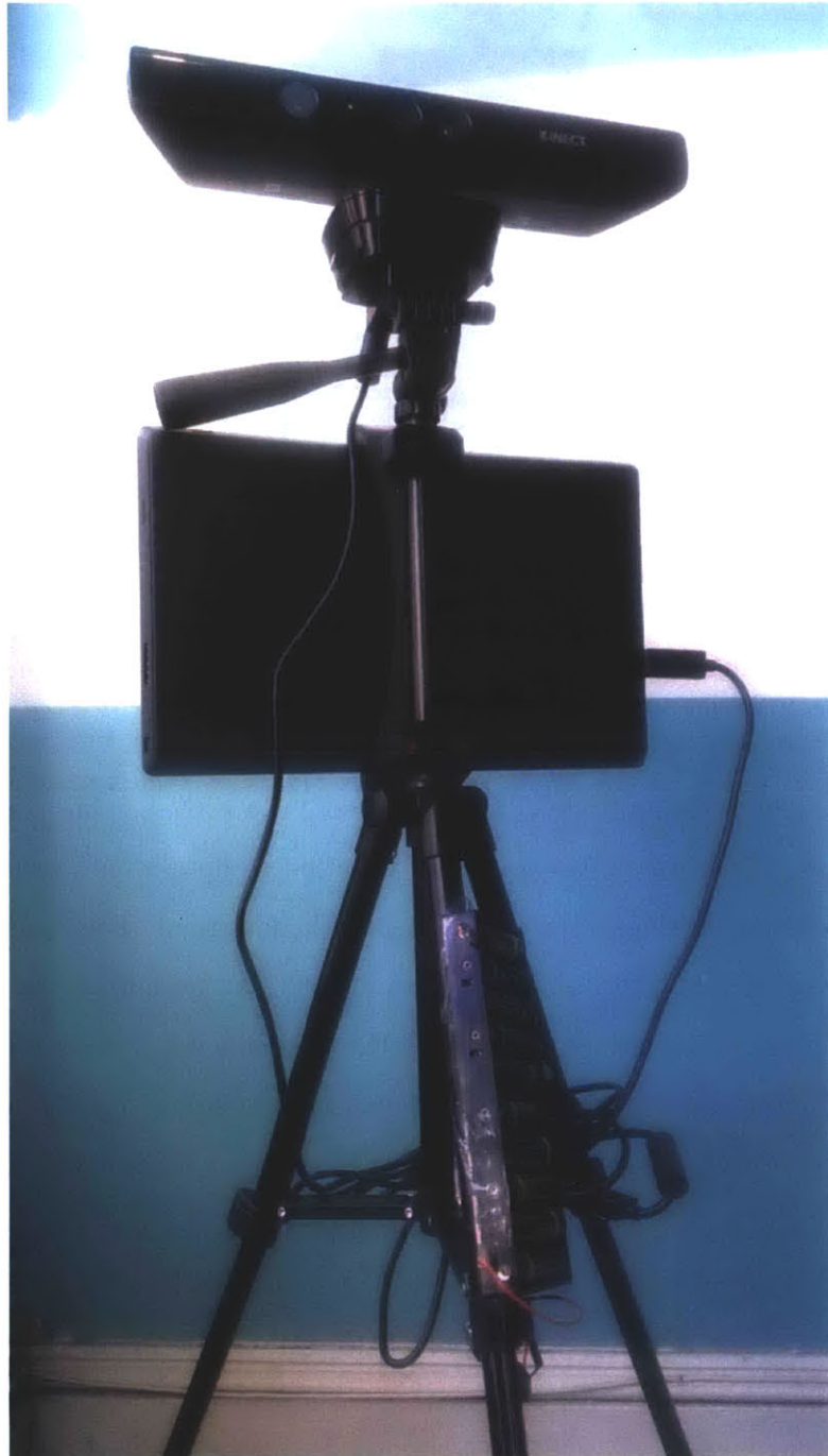
Figure 3-5: EduCase Recorder: Kinect, PC, battery pack, mounted on a tripod
