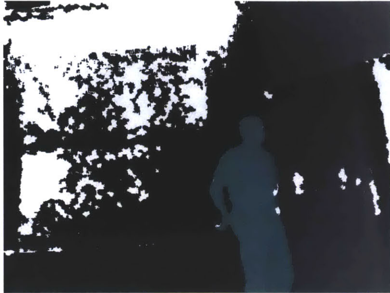
Figure 3-14: The Kinect uses IR light to detect depth. This causes depth data from blackboards appears noisy because black objects absorb infrared light.
