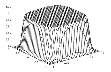
**Figure 5.2.2.** Frequency response magnitude of the tailored two-dimensional spatial filter. The filter specifications, described in Section 5.2.1, were chosen to maximize attenuation near the corners of k-space while preserving the remainder of k-space. The frequency axes are plotted in units of radians divided by pi.
