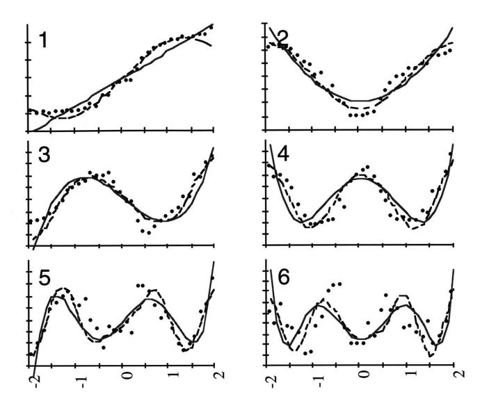
**Figure 5.3.1.** Temporal data representing the first six eigenvectors of the simulated data set (dashed line) and the experimentally observed human data (dots), and the first six terms of the Legendre polynomial model (solid line). X-axis: degrees of rotation.
