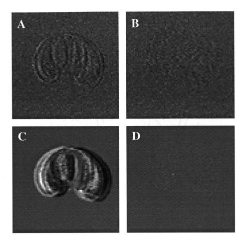
**Figure 4.2.4.** Correction of small and large translations. (A) Difference image for translation of 0.127 pixels. Significant edge-related artifacts are introduced for even small subpixel shifts. (B) Residual difference image after registration of images from (A). (C) Difference image for translation of 5.97 pixels. (D) Residual difference image after registration of images from (C).
