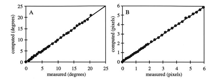
**Figure 4.2.2.** Computed vs. measured displacements for the two imaging phantoms. (A) Rotation. (B) Translation.
