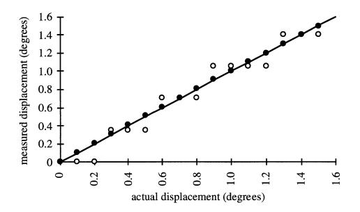
**Figure 4.3.1.** Measured vs. actual rotational displacements for the original DART algorithm (open circles) and the enhanced DART algorithm (solid circles). The enhanced method yields more accurate, continuous estimation of rotational displacements. Perfect solutions lie along the solid line.
