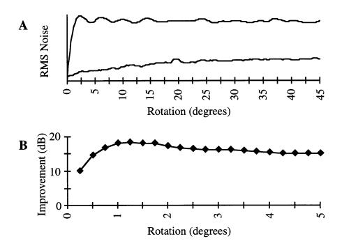
**Figure 4.2.5.** A comparison of errors introduced by linear interpolation and frequency regridding methods. (A) RMS Noise introduced following consecutive clockwise and counterclockwise rotations through the angle specified for linear interpolation (top) and frequency regridding (bottom). (B) Decibel reduction in noise for small rotations provided by frequency regridding.
