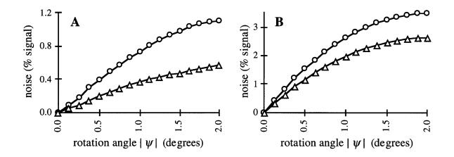
**Figure 5.2.6.** Root mean square difference error, i.e. registration-related noise, as a percentage of the signal vs. rotation angle in simulated images through a perfect cylinder corrected for rotation. Circles: before spatial filtering. Triangles: after spatial filtering. (A) Frequency regridding, average reduction 49.6%. (B) Bilinear interpolation, average reduction 24.5%.
