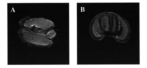
**Figure 4.2.1.** Imaging phantoms used to measure accuracy of the registration algorithm. (A) Representative image of the orange phantom used to assess rotational estimation. (B) Representative image of the tomato phantom used to assess translational estimation.
