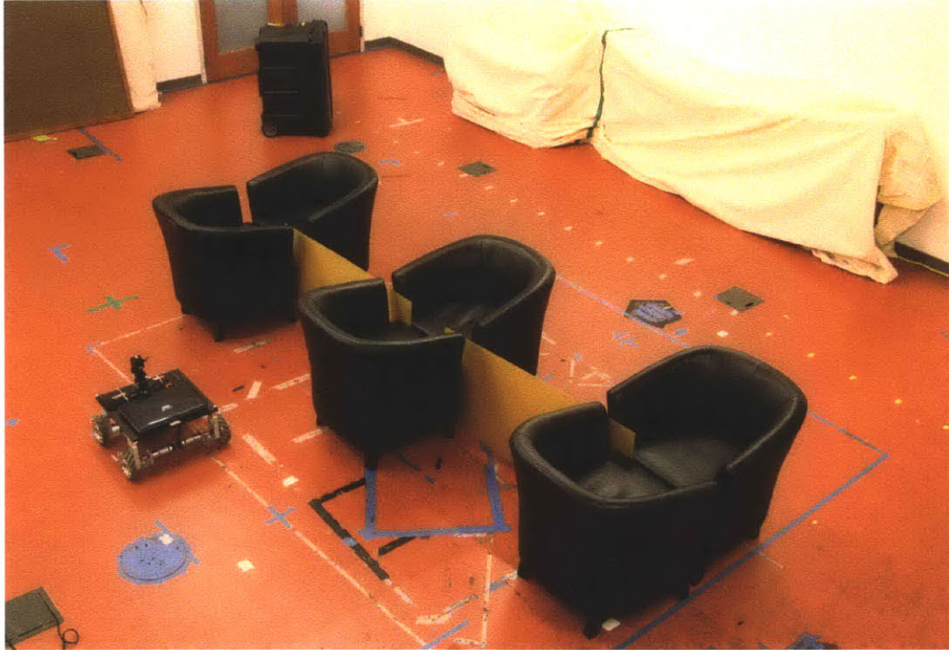
Figure 4-6: An omnidirectional ground robot with 360 degree laser rangefinder is driven clockwise around a center opaque barrier for the occupancy grid mapping experiment. The hardware experiment in Section 4.4.3 employing a SLAM algorithm uses the same robot system within a different environment.
