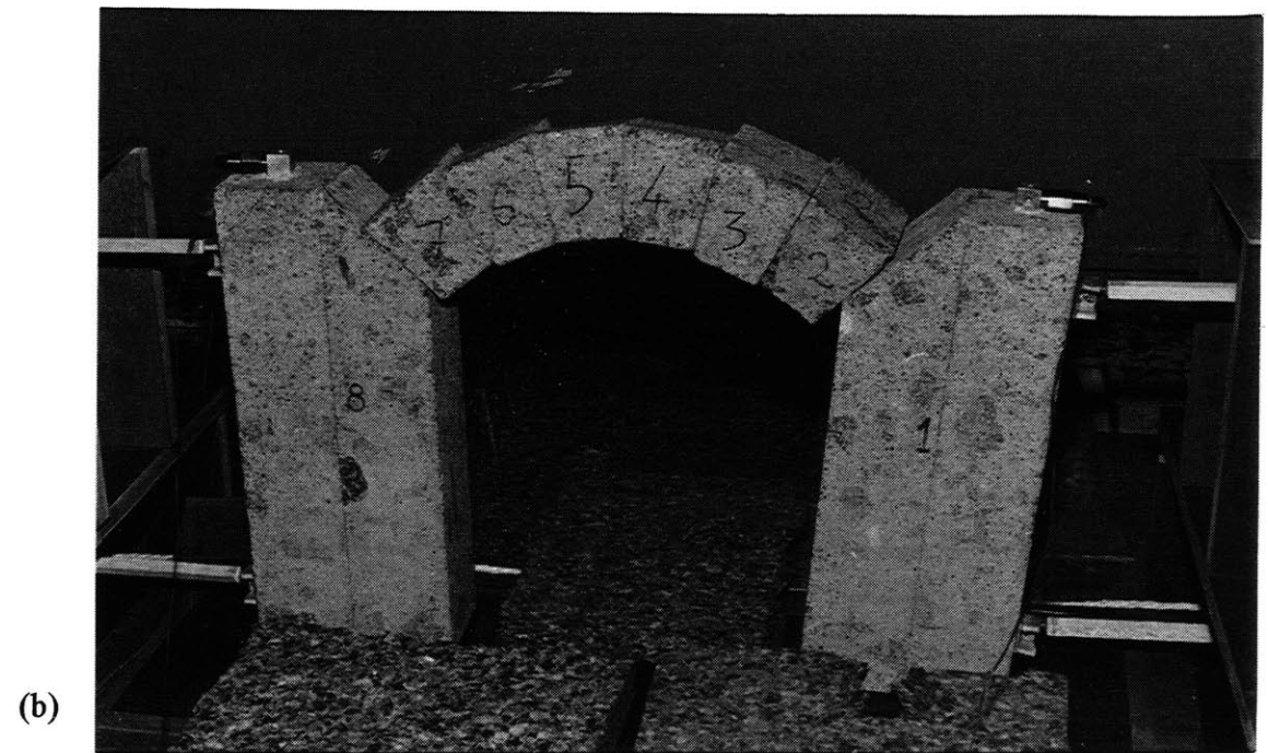
Figure 6-6. (a) Instrumented arch model on shaking table; (b) Displaced arch configuration after a test.
