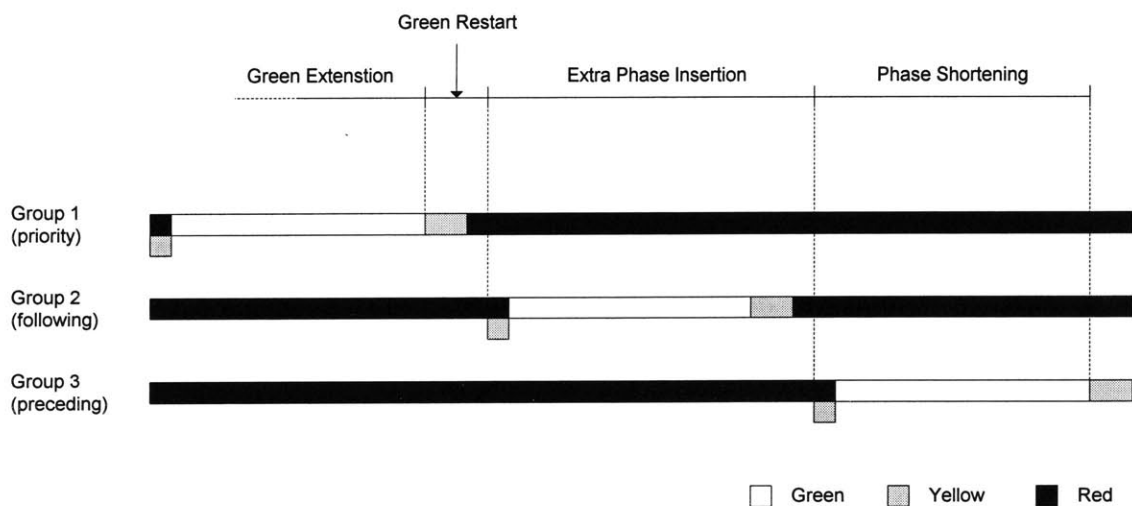
Figure 6-1: PRIBUSS priority actions during a typical 3-phase cycle (source: Davol, 2001)
