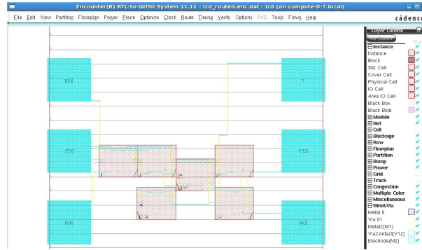
Figure 6.3. A placed and routed LZD2 circuit in the scaled 6T process technology, whose physical data is scaled to the predictive 90nm equivalent 6T NEM relays process technology and used alongside a predictive 90nm equivalent 6T NEM relays process interconnect capacitance table file to estimate post-route switching power.
