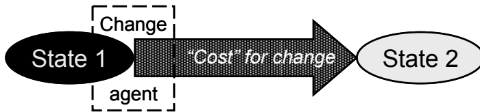
Figure 1. Change defined as state transition. Change specifications must include descriptions of beginning state 1, ending state 2, change mechanism including cost, and the change agent instigating the change.
