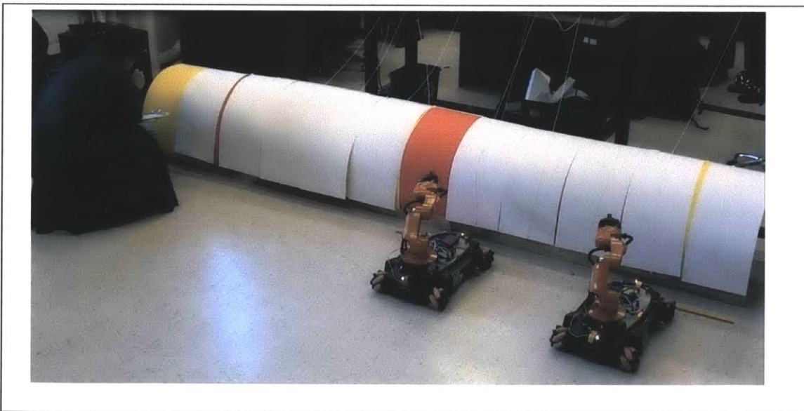
Figure 5-6: Hardware demonstration of Tercio. Two KUKA Youbots build a mock airplane fuselage. A human worker requests time on the left half of the fuselage to perform a quality assurance inspection, and the robots replan.
