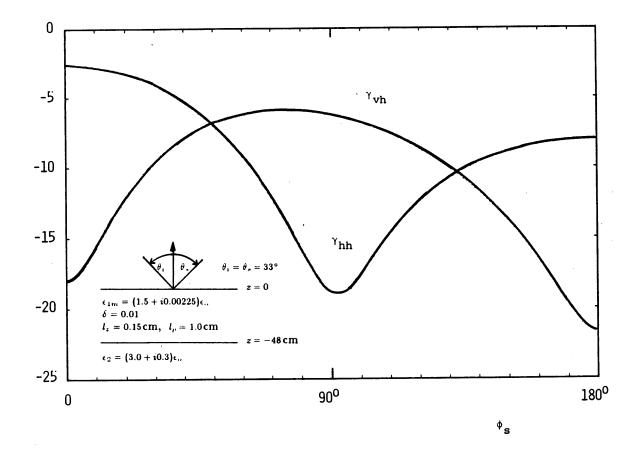
Figure 7.8 Bistatic scattering coefficients  $\gamma_{hh}$  and  $\gamma_{vh}$  as a function of azimuthal scattering angle  $\phi_s$  at 10 GHz.
