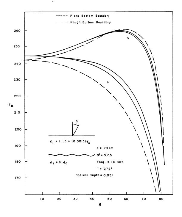
Figure 9.2 Brightness temperature as a function of angle for rough surface at bottom boundary.
