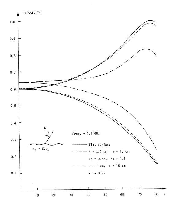
Figure 4.1 Emissivities as a function of observation angle – Modified Small Perturbation Method.
