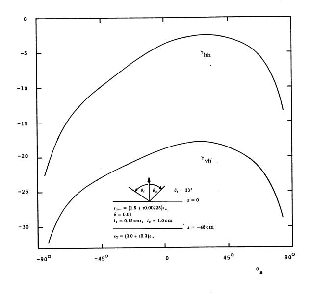
Figure 7.5 Bistatic scattering coefficients  $\gamma_{hh}$  and  $\gamma_{vh}$  as a function of scattering angle  $\theta_s$  at 10 GHz.
