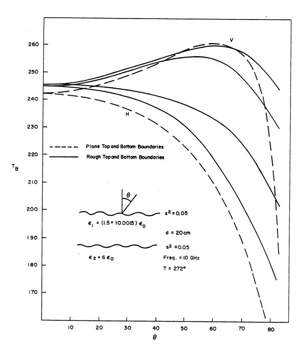
Figure 9.8 Brightness temperature as a function of angle for rough surfaces at top and bottom boundaries.
