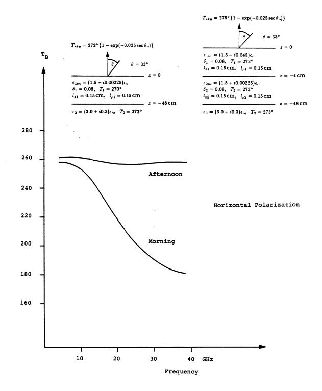
Figure 6.7 Brightness temperature as a function of frequency for a three-layer random medium.
