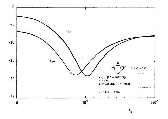
Figure 7.9 Bistatic scattering coefficients  $\gamma_{hh}$  and  $\gamma_{vv}$  as a function of azimuthal scattering angle  $\phi_{s}$  at 10 GHz.
