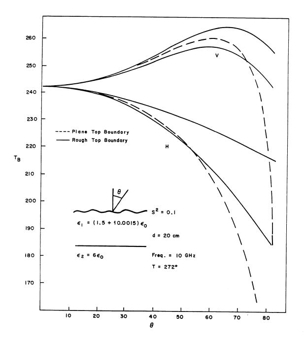
Figure 9.7 Brightness temperature as a function of angle for rough surface at top boundary with  $s^2 = 0.1$ .
