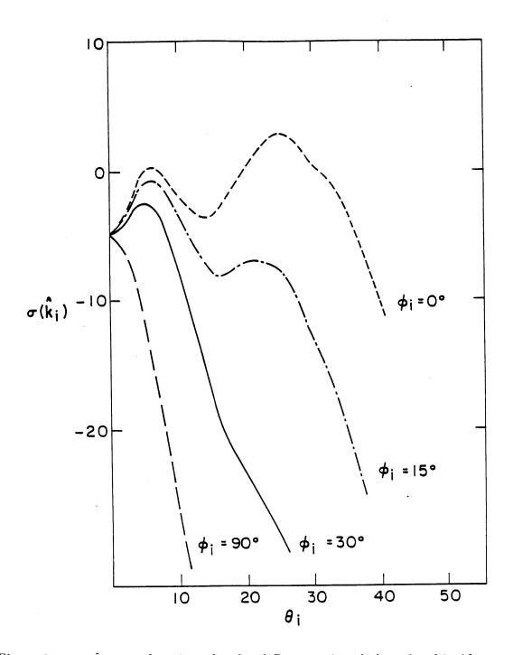
Figure 5.5  $\sigma(\hat{k}_i)$  as a function of  $\theta_i$  for different azimuthal angle of incidence  $\phi_i$  at 1.4 GHz with  $\sigma = 1$  cm, l = 50 cm. B = 10 cm, P = 100 cm,  $\sigma_x = 0$ , and  $\epsilon_1 = (6.0 + i0.6)\epsilon_{ii}$ .
