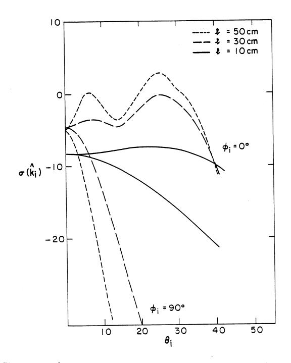
Figure 5.4  $\sigma(\hat{k}_i)$  as a function of  $\theta_i$  for different values of l at 1.4 GHz with  $\sigma = 1$  cm, B = 10 cm, P = 100 cm,  $\sigma_x = 0$ , and  $\epsilon_1 = (6.0 + i0.6)\epsilon_0$ .
