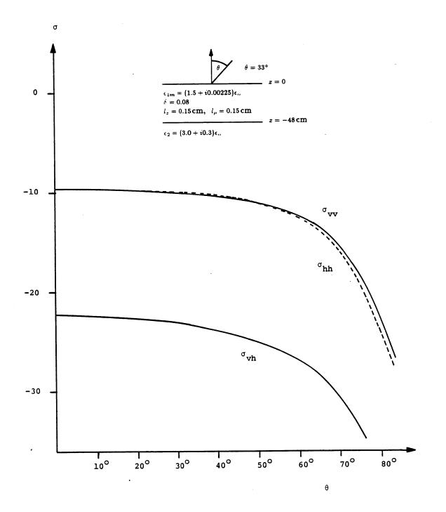
Figure 7.3 Backscattering cross sections as a function of incident angle at 10 GHz.
