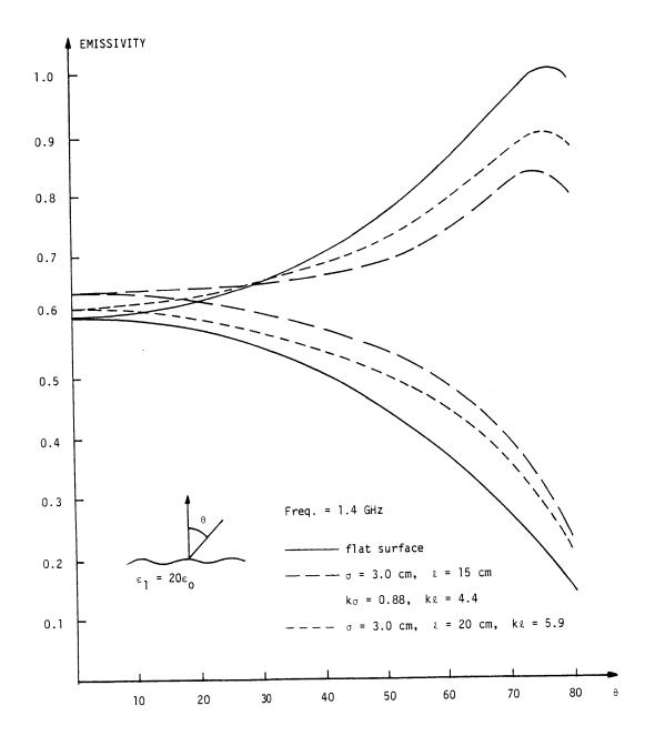
Figure 4.3 Emissivities as a function of observation angle – Modified Small Perturbation Method.
