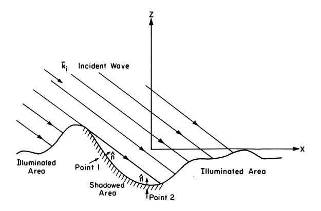
Figure 2.2 The shadowed area on the rough surface.
