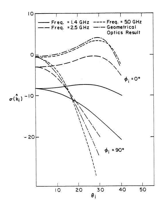
Figure 5.2  $\sigma(\hat{k}_i)$  as a function of  $\theta_i$  for different frequencies with  $\sigma = 1$  cm, l = 10 cm, B = 10 cm, P = 100 cm,  $\sigma_x = 0$ , and  $\epsilon_1 = (6.0 + i0.6)\epsilon_{ij}$ .
