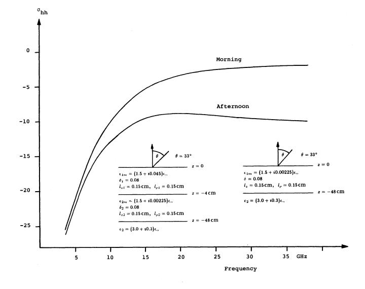
Figure 8.2 Backscattering cross section for horizontally polarized like-like return  $\sigma_{hh}$ as a function of frequency for a three-layer random medium.
