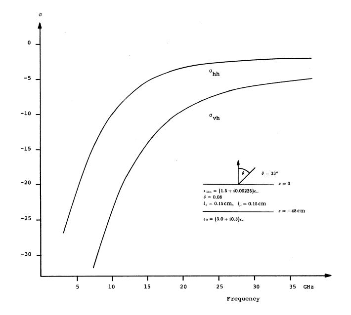
Figure 7.2 Backscattering cross sections as a function of frequency.
