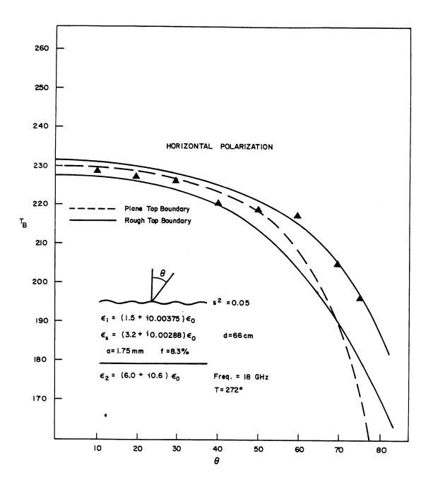
Figure 9.13 Brightness terperature as a function of angle at 18 GHz for horizontal polarization.
