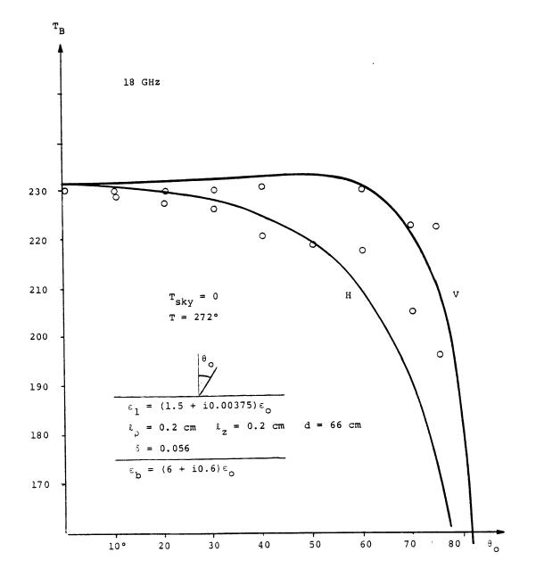
Figure 6.5 Brightness temperature as a function of observation angle at 18 GHz.
