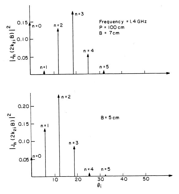
Figure 5.7 (b) Locations and amplitudes of the modes for B = 7 cm and B = 5 cm.
