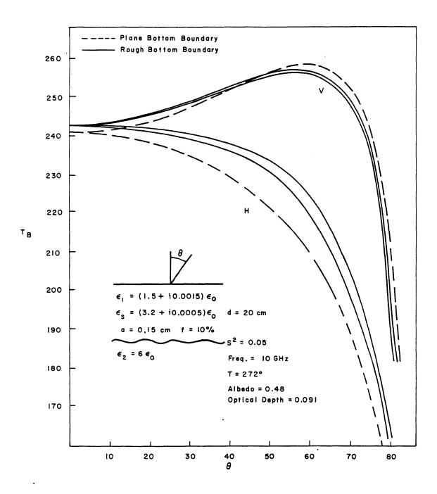
Figure 9.9 Brightness temperature as a function of angle for rough surface at bottom boundary with volume scattering.
