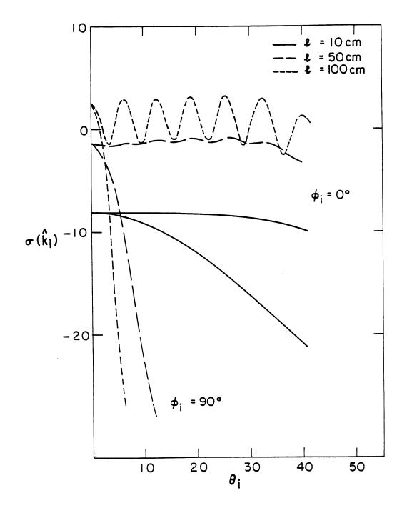
Figure 5.11  $\sigma(\hat{k}_i)$  as a function of  $\theta_i$  for different values of l at 1.4 GHz with  $\sigma = 1$  cm, B = 10 cm, P = 100 cm,  $\sigma_x = 5$  cm,  $l_x = 300$  cm, and  $\epsilon_1 = (6.0 + i0.6)\epsilon_{ii}$ .
