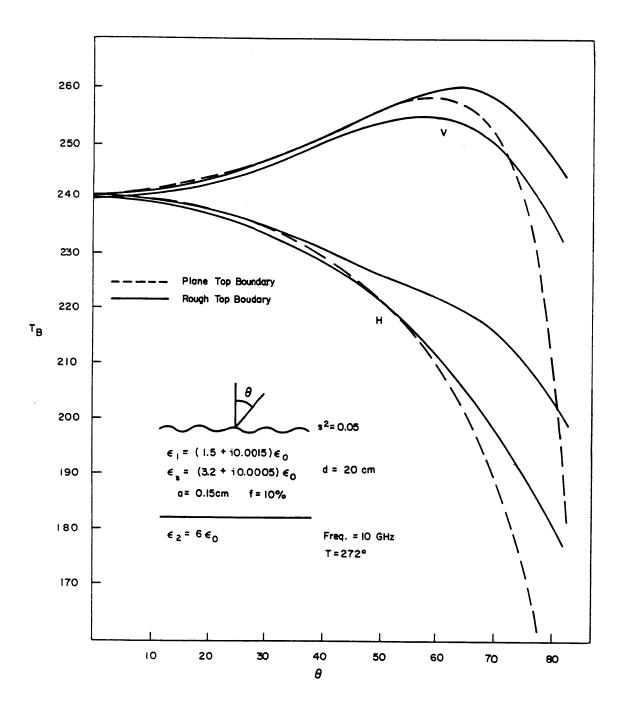
Figure 9.10 Brightness temperature as a function of angle for rough surface at top boundary with volume scattering.
