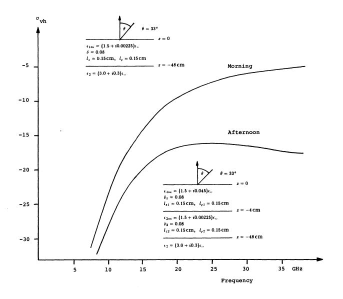
Figure 8.3 Backscattering cross section for depolarized return  $\sigma_{vh}$  as a function of frequency for a three-layer random medium.
