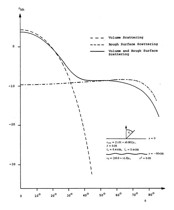
Figure 10.3 Backscattering cross sections as a function of incident angle for volume scattering, rough surface scattering, and combined volume and rough surface scattering at 5 GHz.
