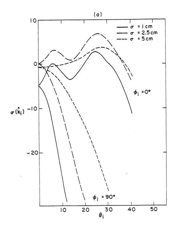
Figure 5.9 (a)  $\sigma(\hat{k}_i)$  as a function of  $\theta_i$  for different values of  $\sigma$  at 1.4 GHz with l = 50 cm, B = 10 cm, P = 100 cm,  $\sigma_x = 0$ , and  $\epsilon_1 = (6.0 + i0.6)\epsilon_{ij}$ .
