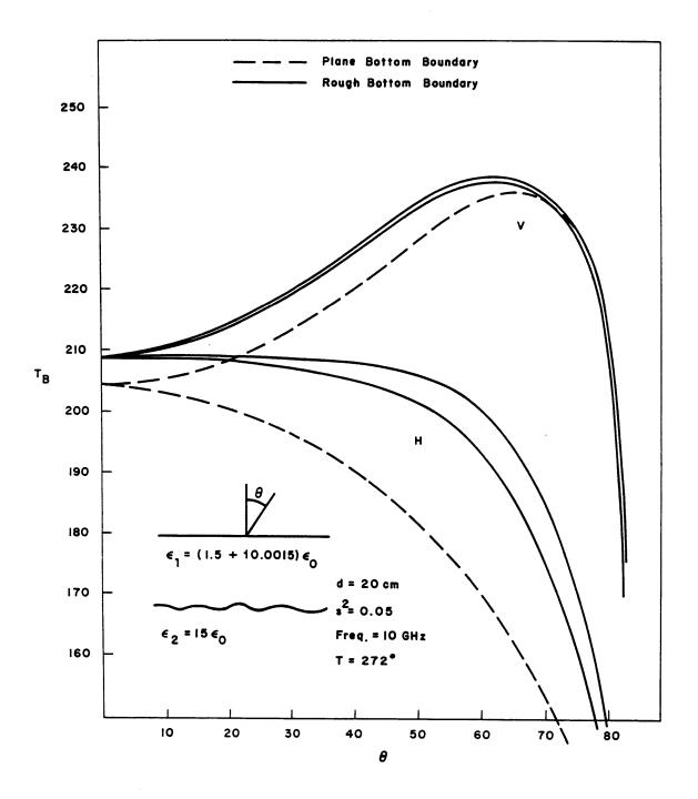
Figure 9.3 Brightness temperature as a function of angle for rough surface at bottom boundary with  $\epsilon_2 = 15\epsilon_{,n}$ .
