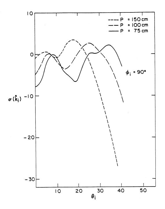
Figure 5.8  $\sigma(\hat{k}_i)$  as a function of  $\theta_i$  for different values of P at 1.4 GHz with  $\sigma = 1$  cm. l = 50 cm, B = 10 cm, P = 100 cm,  $\sigma_x = 0$ , and  $\epsilon_1 = (6.0 + i0.6)\epsilon_0$ .
