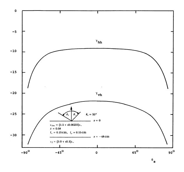
Figure 7.4 Bistatic scattering coefficients  $\gamma_{hh}$  and  $\gamma_{vh}$  as a function of scattering angle  $\theta_s$  at 10 GHz.
