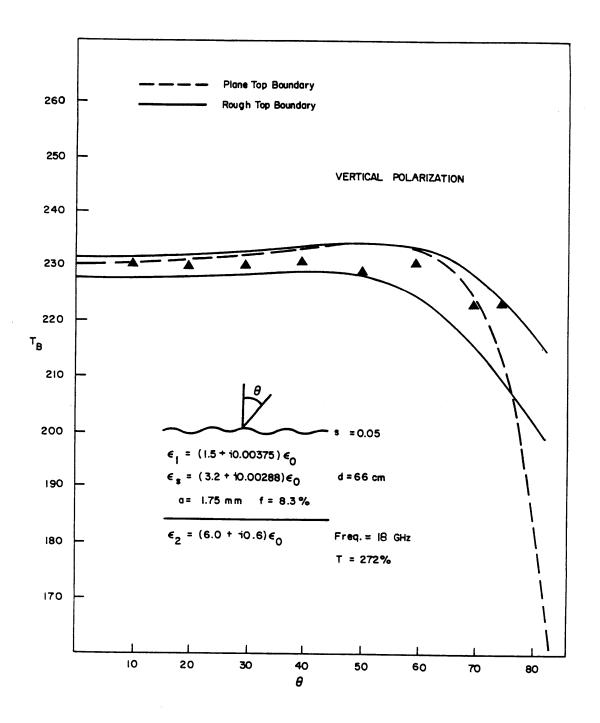
Figure 9.12 Brightness temperature as a function of angle at 18 GHz for vertical polarization.
