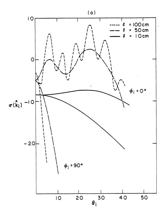
Figure 5.6 (a)  $\sigma(\hat{k}_i)$  as a function of  $\theta_i$  for different values of l at 1.4 GHz with  $\sigma = 1$  cm, B = 10 cm, P = 100 cm,  $\sigma_x = 0$ , and  $\epsilon_1 = (6.0 + i0.6)\epsilon_{ij}$ .
