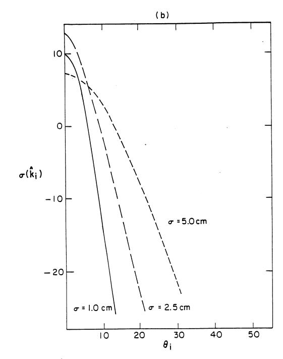
Figure 5.9 (b)  $\sigma(\hat{k}_i)$  as a function of  $\theta_i$  for different values of  $\sigma$  at 1.4 GHz with l = 50 cm, B = 0,  $\sigma_x = 0$ , and  $\epsilon_1 = (6.0 + i0.6)\epsilon_{ii}$ .
