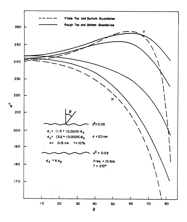
Figure 9.11 Brightness temperature as a function of angle for rough surface at top and bottom boundaries with volume scattering.
