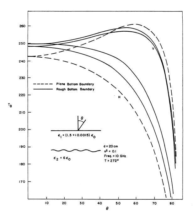
Figure 9.4 Brightness temperature as a function of angle for rough surface at bottom boundary with  $s^2 = 0.1$ .
