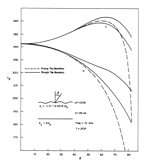
Figure 9.6 Brightness temperature as a function of angle for rough surface at top boundary.
