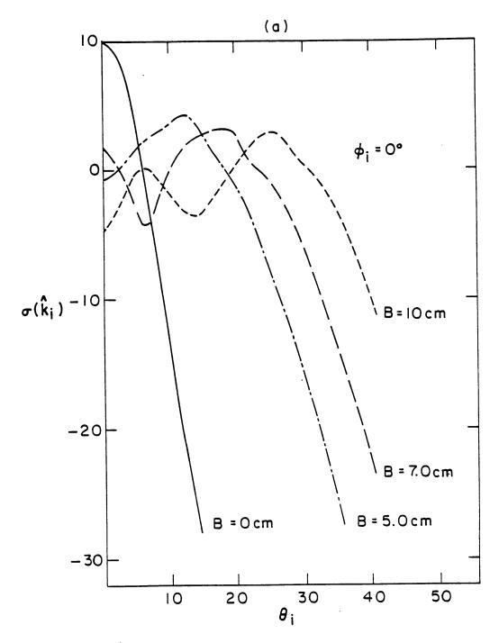
Figure 5.7 (a)  $\sigma(\hat{k}_i)$  as a function of  $\theta_i$  for different values of B at 1.4 GHz with  $\sigma = 1 \text{ cm}, l = 50 \text{ cm}, P = 100 \text{ cm}, \sigma_J = 0, \text{ and } \epsilon_1 = (6.0 + i0.6)\epsilon_0$ .
