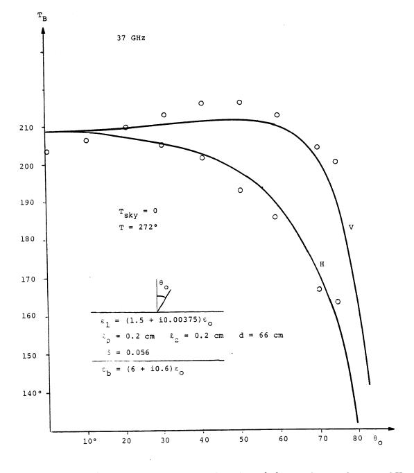
Figure 6.6 Brightness temperature as a function of observation angle at 37 GHz.
