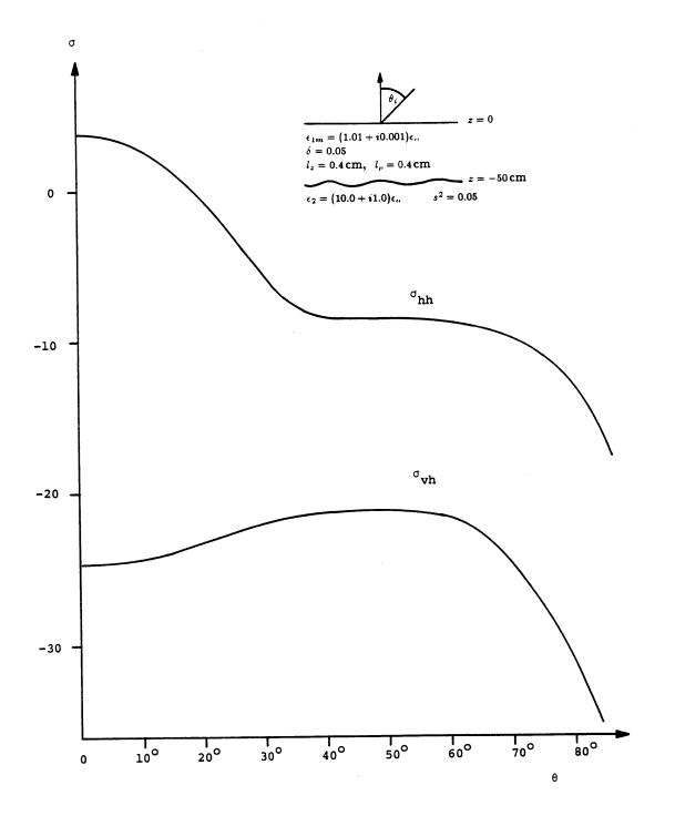
Figure 10.2 Backscattering cross sections as a function of incident angle for rough surface and volume scattering at 5 GHz.
