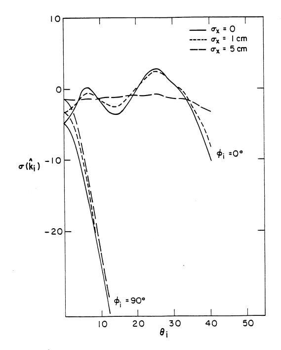
Figure 5.12  $\sigma(\hat{k}_i)$  as a function of  $\theta_i$  for different values of  $\sigma_x$  at 1.4 GHz with  $\sigma = 1$ cm, l = 50 cm, B = 10 cm, P = 100 cm,  $l_x = 300$  cm, and  $\epsilon_1 = (6.0 + i0.6)\epsilon_{obc}$ .
