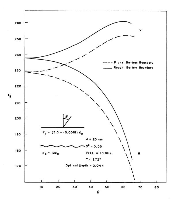
Figure 9.5 Brightness temperature as a function of angle for rough surface at bottom boundary with  $\epsilon_1 = (3.0 + i0.0018)\epsilon_{...}$
