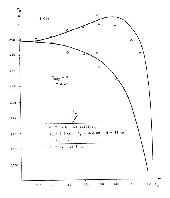
Figure 6.3 Brightness temperature as a function of observation angle at 5 GHz.
