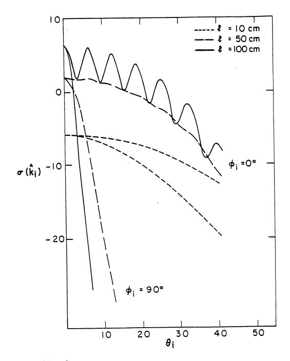
Figure 5.10 (a)  $\sigma(\hat{k}_i)$  as a function of  $\theta_i$  for different values of l at 1.4 GHz with  $\sigma = 1 \text{ cm}$ , B = 0, P = 100 cm,  $\sigma_x = 5 \text{ cm}$ ,  $l_x = 300 \text{ cm}$ , and  $\epsilon_1 = (6.0 + i0.6)\epsilon_{in}$ .
