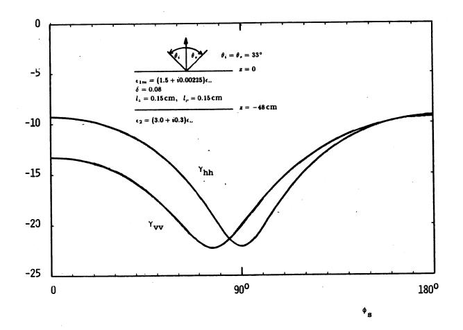
Figure 7.7 Bistatic scattering coefficients  $\gamma_{hh}$  and  $\gamma_{vv}$  as a function of azimuthal scattering angle  $\phi$ , at 10 GHz.
