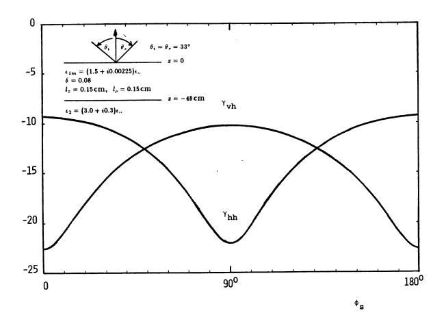
Figure 7.6 Bistatic scattering coefficients  $\gamma_{hh}$  and  $\gamma_{vh}$  as a function of azimuthal scattering angle  $\phi_s$  at 10 GHz.
