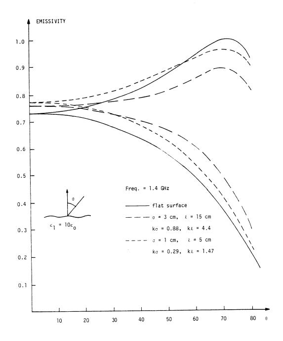
Figure 4.5 Emissivities as a function of observation angle – Modified Small Perturbation Method.
