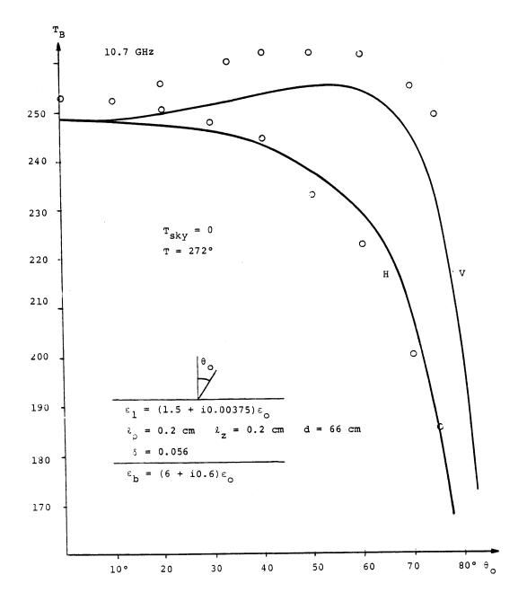
Figure 6.4 Brightness temperature as a function of observation angle at 10.7 GHz.
