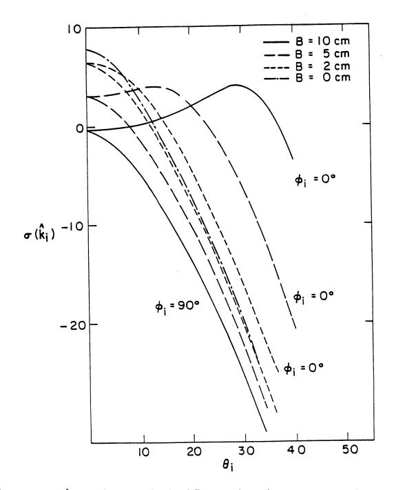
Figure 5.3  $\sigma(\hat{k}_i)$  as a function of  $\theta_i$  for different values of *B* at 5.0 GHz with P = 100 cm,  $\sigma = 1$  cm, l = 10 cm,  $\sigma_x = 0$ , and  $\epsilon_1 = (6.0 + i0.6)\epsilon_{ij}$ .
