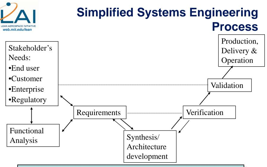
Systems engineering process is applied at multiple levels: system, subsystem, component.
