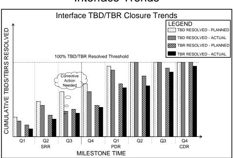
**Interface TBD/TBR Closure Trends.** The graph illustrates the actual cumulative number of TBDs and TBRs that have been resolved compared to what is planned to be resolved based on historical data and expectations given the program characteristics. It can be seen that in Q3 after SRR, the actual TNDs are
