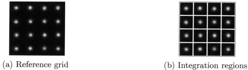
Figure 6-1: Reference grid and integration superpixels for CCD imaging. The image used above are (background-subtracted) superposition of the measurements of all 64 symbols, in order to produce a reference for the relative locations of all 16 FB modes at the CCD plane. The boundaries of the superpixel partitions are shown as white lines (inclusive) in Figure 6-1b, which is otherwise the same image.
