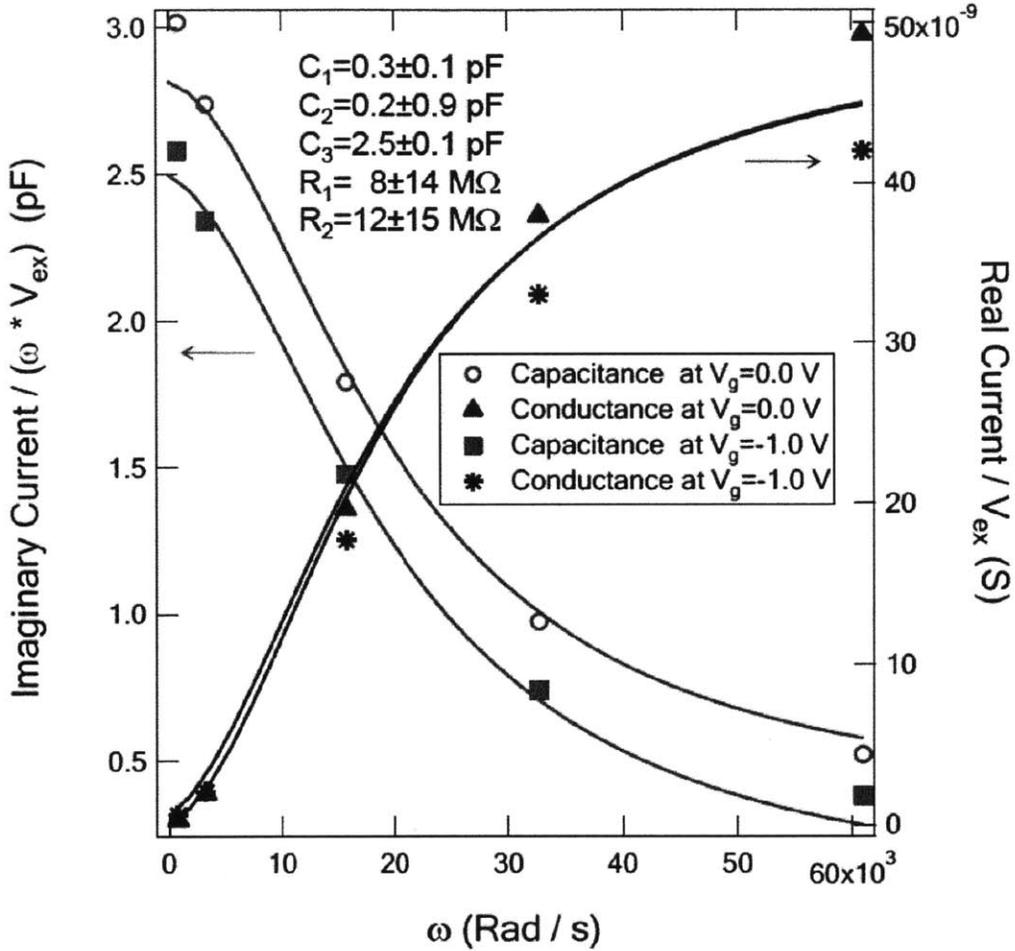
Figure 3-5: Fits of current as a function of frequency using the circuit model depicted in Figure 3-4. As we can see, there is a decent agreement in the fit and the experimental data. The value of  $C_1 = 0.3 \pm 0.1 \text{ pF}$ , which corresponds to the capacitance between the gate and the 2DEG matches up quite nicely with the theoretically expected value of  $0.32 \text{ pF}$ . Figure taken from [26]
