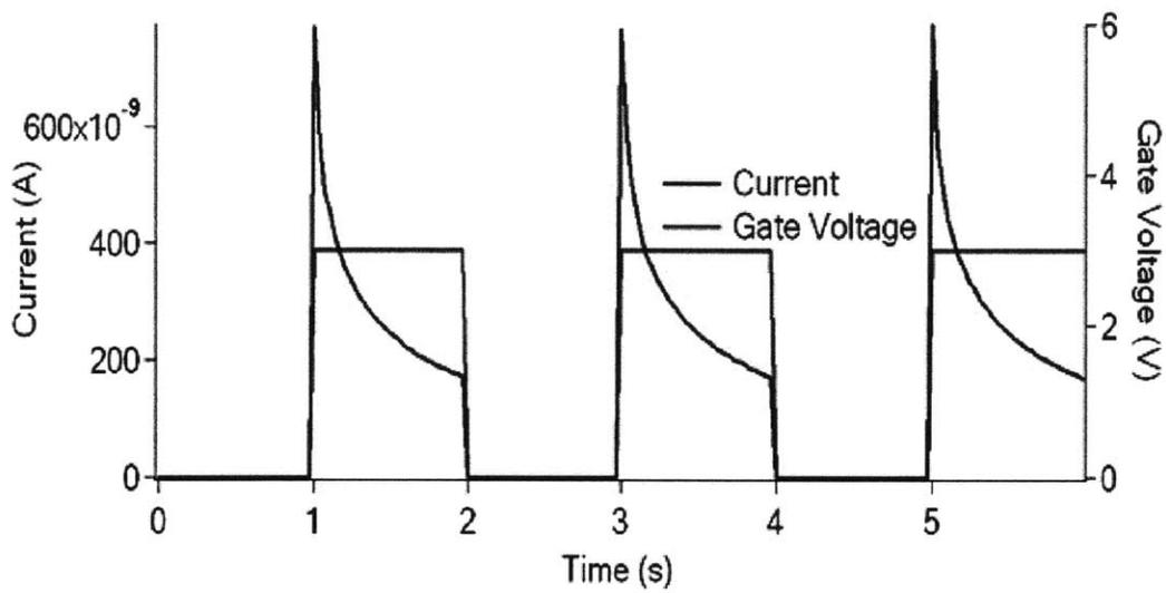
Figure 4-4: Evidence of possible charge trapping in the oxide layer. Here, the DC current is measured between a pair of ohmics, while the gate voltage on the top gate is changed from 0 V to 3 V. Immediately, a current appears, however, this current exponentially decays as a function of time. A possible explanation for this exponential decay in current is charge trapping in the oxide layer.
