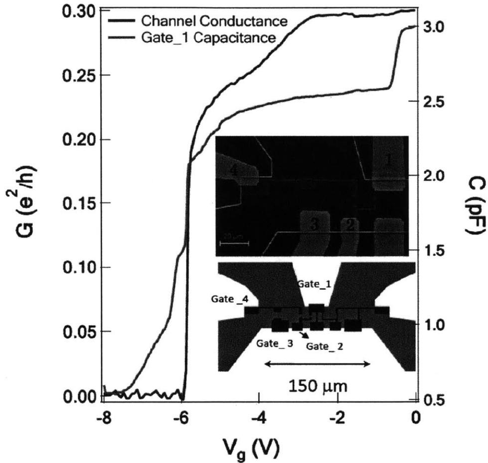
Figure 3-2: a) A negative DC bias is applied to gate 2, and the capacitance of the gate with the underlying 2DEG, and the conductance of the 2DEG are measured. An initial drop in the capacitance occurs at around  $V_g = -0.4$  V, and this drop is equal to the theoretically calculated capacitance of gate 2. As the negative bias is increased in magnitude, around -6 V, both the capacitance and conductance drop to zero, indicating that the 2DEG has been completely depleted. Figure taken from [26]
