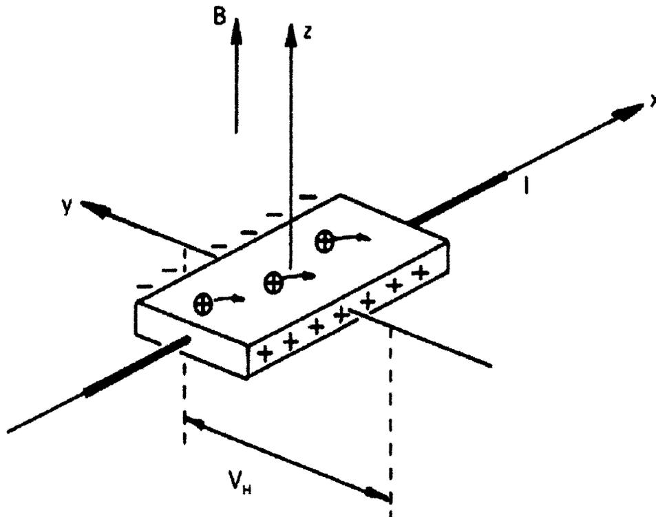
Figure 1-3: Classical Hall Effect. A current is passed through the sample, with a magnetic field perpendicular to the current. Due to the Lorentz force from the magnetic field, a voltage transverse to both the current and the field develops, known as the Hall Voltage. Figure taken from reference [18]
