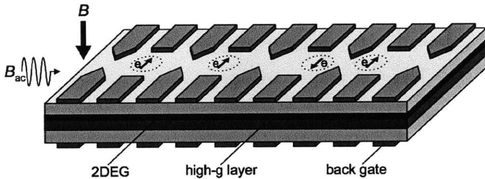
Figure 1-7: The implementation of a quantum computer using the spin of quantum dots. Here, lateral gates are used to deplete the 2DEG underneath, forming quantum dots. Electrical pulses are applied on the tunnel barrier of between each dots for two-qubit operations, while a pulsing magnetic field B is used to perform single qubit operations. Figure from [24]
