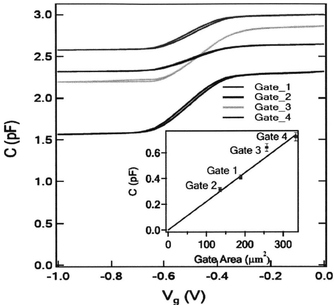
Figure 3-3: Capacitance measurements of each gate, as a function of gate voltage applied. As the magnitude of  $V_g$  is increased, there is a corresponding drop in the capacitance. This experimental drop matches up quite nicely with the theoretical capacitance of each gate. Figure taken from [26]
