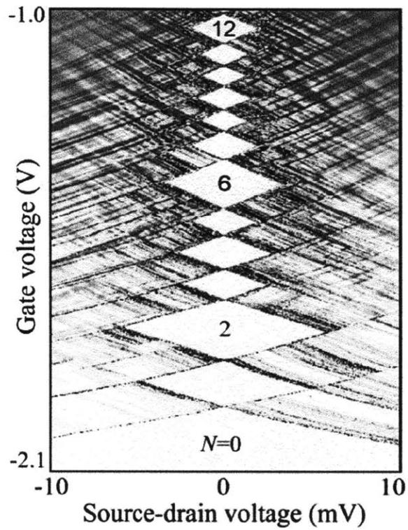
Figure 1-6: An example of coulomb blockade diamonds. The diamonds in the center each correspond to having a discrete number of electrons in the dot, with  $N=0$  for the diamond at the bottom, and  $N=12$  for the diamond at the top. Image taken from reference [22]
