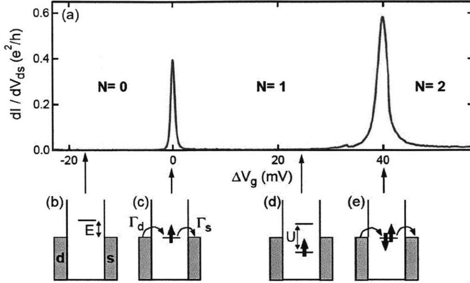
Figure 1-5: An example of coulomb blockade in a quantum dot. Conductance is plotted as a function of gate voltage, with  $V_{\text{source}} = V_{\text{drain}}$ . Image taken from reference [21]
