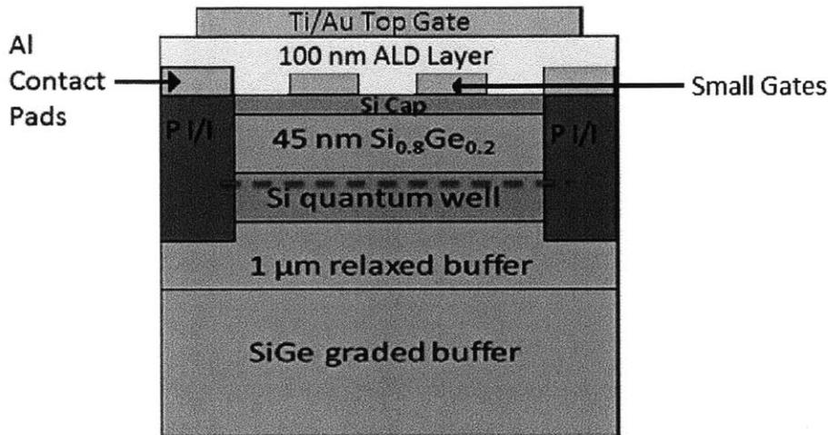
Figure 4-1: Side view schematic of devices fabricated in a undoped Si/SiGe heterostructure
