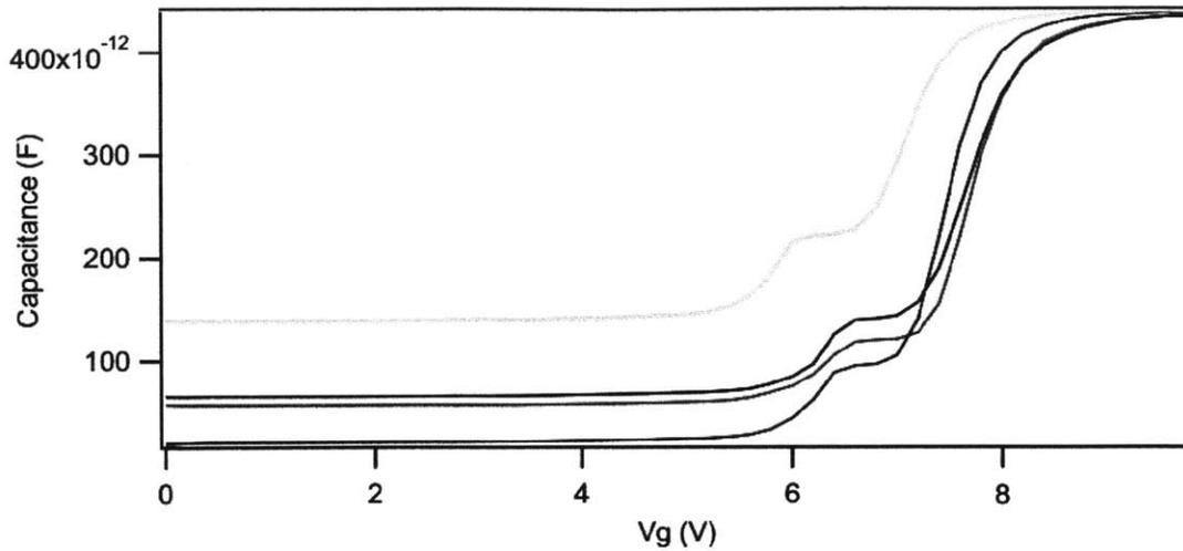
Figure 4-3: Capacitance measurements of devices fabricated with an undoped heterostructure. The capacitance is measured between the metallic top gate, and one of the ohmics. From the data, it appears that initially, there are electrons populating the Si quantum well; however, as the gate voltage is increased, the electrons move very quickly to populate the Si cap layer instead.
