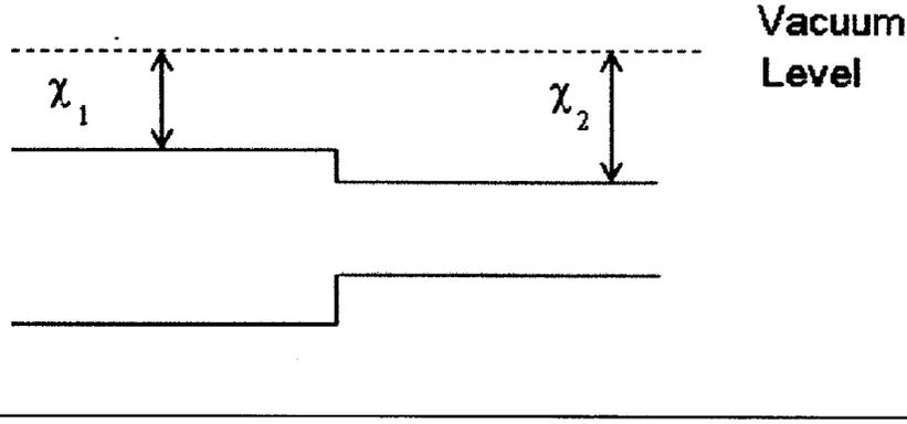
Figure 1-1: Here, we have two semiconductors with different band gaps. At the heterojunction, the conduction and valence bands will line up such that the vacuum levels of both semiconductors match, resulting in a discontinuity for both bands. In this figure,  $\chi_1$ , and  $\chi_2$  are the electron affinities of each semiconductor.
