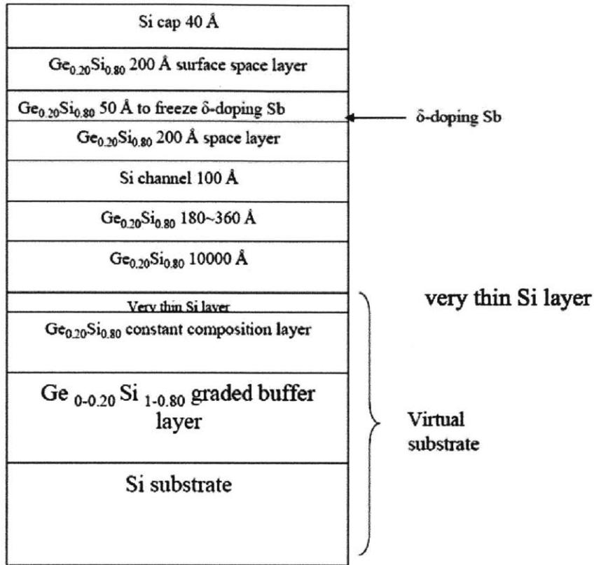
Figure 2-1: An example of a doped Si/SiGe heterostructure. This particular sample was grown by the research group of Professor Ya-Hong Xie. The undoped heterostructures used in this research were similar to the one above, but without a delta doping layer in the spacer SiGe layer above the Si quantum well. Figure taken from [12]
