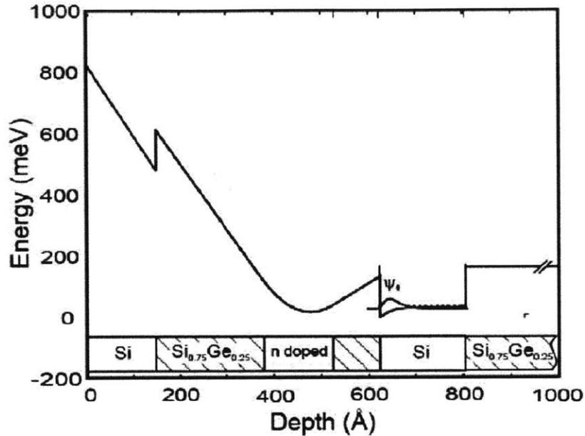
Figure 1-2: The electronic band structure of a modulation doped Si/SiGe heterostructure. The quantum well is at depth of 600 - 800 Å, and the doping occurs between 400-500 Å. Note that there is a dip in the electronic band structure around the doping. If the doping concentration is too high, a parallel conduction band can occur here. Image taken from reference[16]
