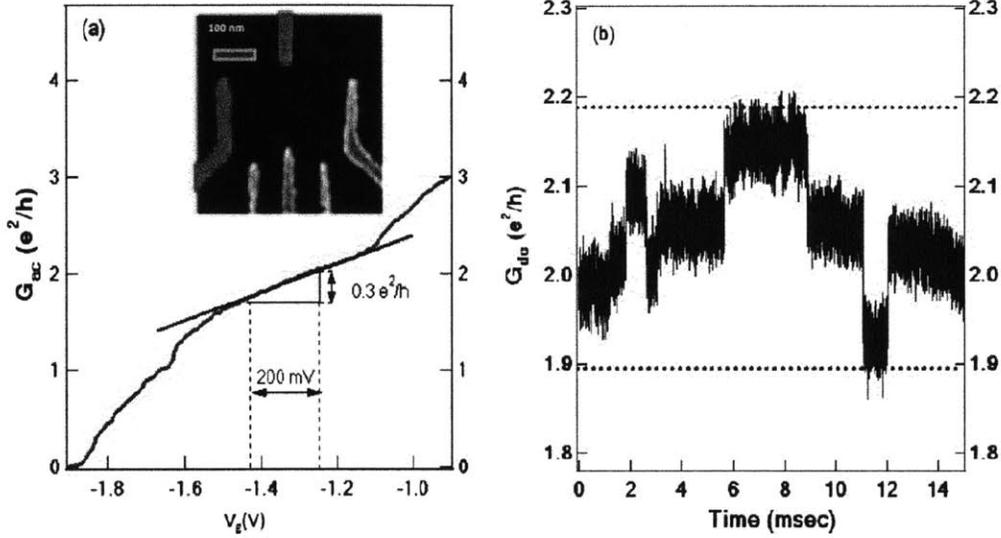
Figure 3-1: a) Conductance through the channel, with negative bias applied to a pair of gates, forming a QPC. (b) Telegraph noise of magnitude  $0.3 e^2/h$ . measured at  $V_g = -1.3 \text{ V}$ , with a bandwidth from 0 - 300 kHz. Figure taken from [26]
