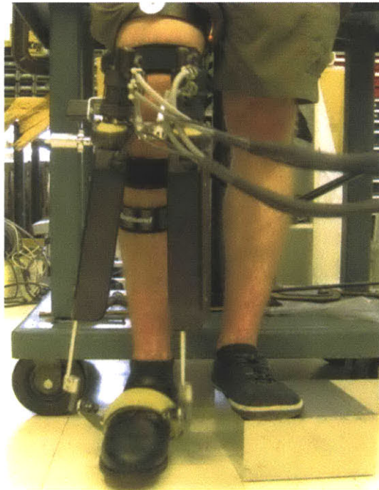
Figure 1. The Anklebot and knee brace were attached on a subject in a standing position with the dominant foot clear of the ground.
