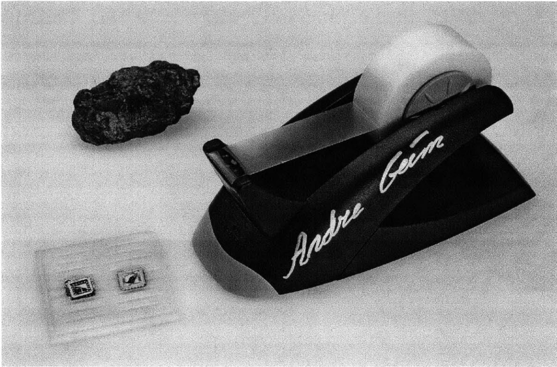
Figure 2.1: A piece of Graphite, A roll of Scotch Tape Signed by Andre Geim, and a graphene transistor. 1
