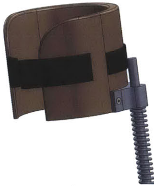
Figure 11: Computer rendering of an attachment mechanism for a compression spring.
