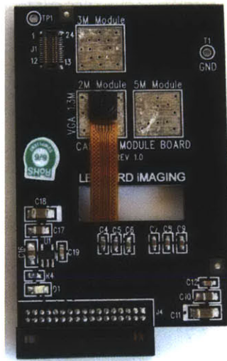
Figure 3-4: Picture of a Leopard Imaging LI-LIBCMVGA Camera Module [16].
