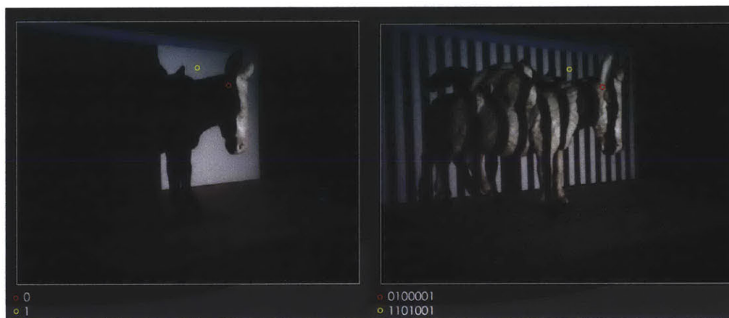
Figure 2.3: Example of light stripe sequence progression. Each pixel is assigned a gray code signature of 1s and 0s, which is used to calculate the distance of that pixel from the camera [9].
