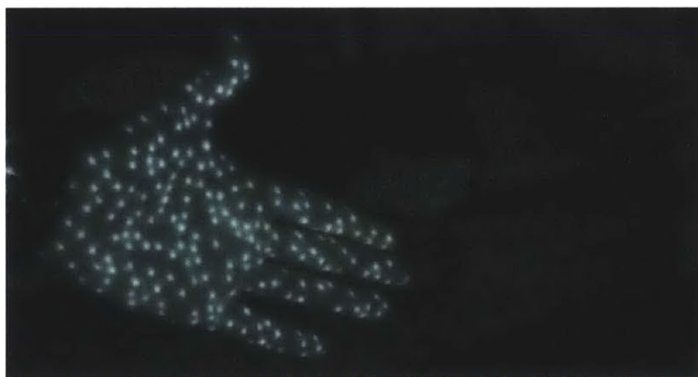
Figure 1-4: Example of Xbox Kinect projection pattern and distortions [6].
