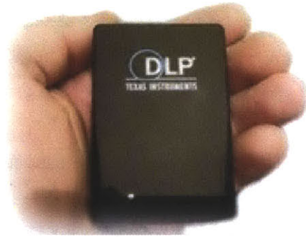
Figure 3-5: Picture of a TI Pico Projector Development Kit [8].
