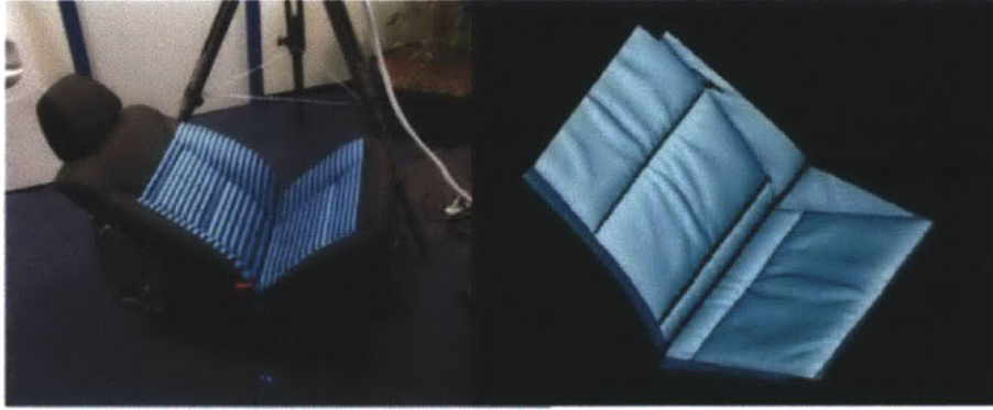
Figure 2.4: Example of structured light used to model automotive applications [12].
