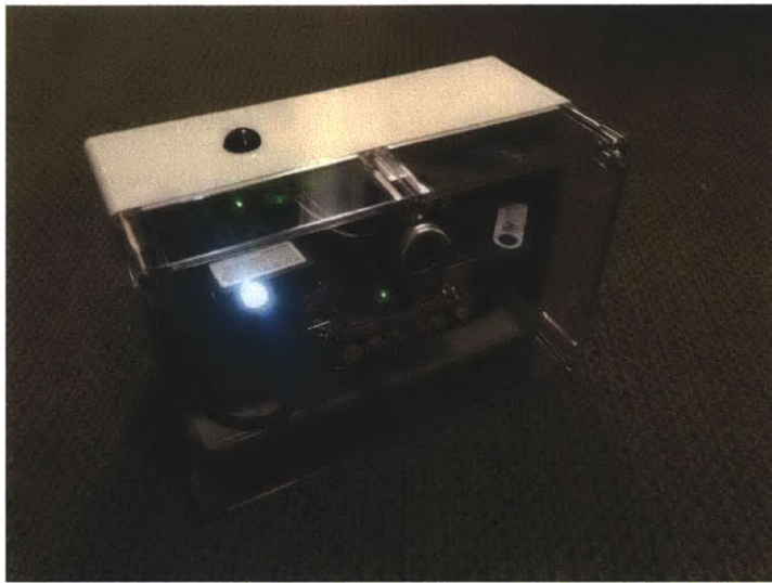
Figure 3-7: Completed underwater structured light 3-D imaging system.
