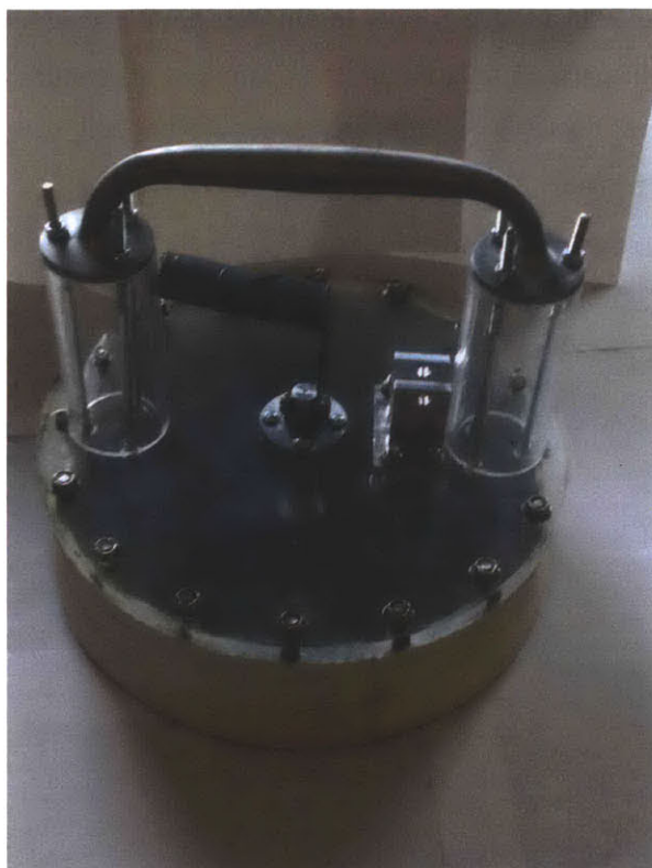
Figure 13: The gripper assembled with the skirt and the simple actuator
