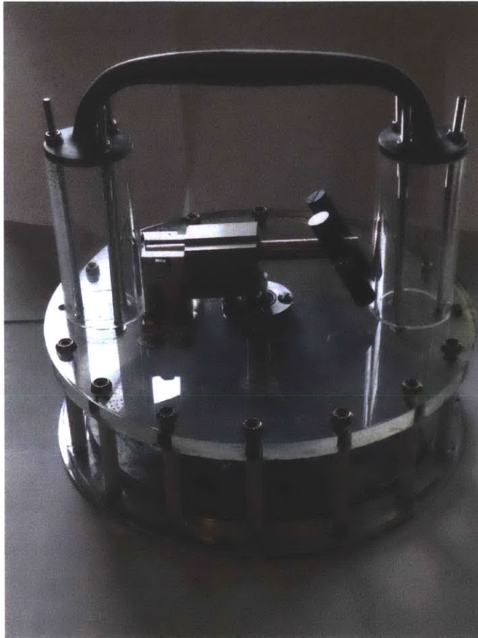
Figure 12: The gripper assembled without the skirt (the skirt is the part that keeps ferrofluids from getting inside the housing)
