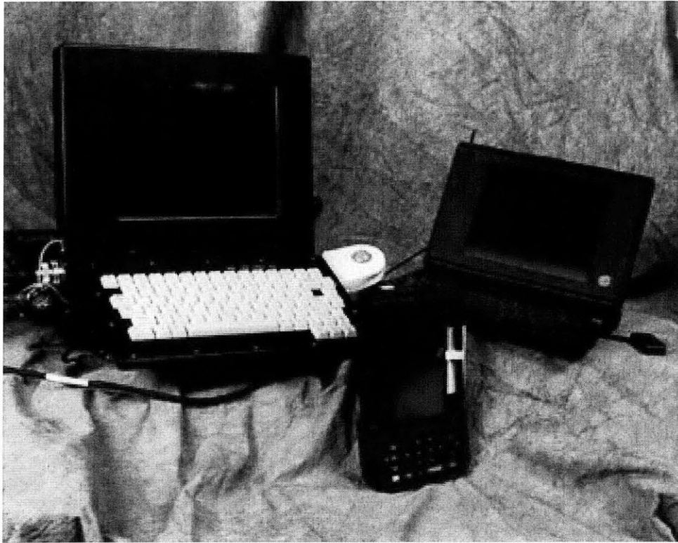
Figure 3.2: WNE (computers) components, left to right: Wireless Network Server (WNS); NORAND PenKey Personal Digital Assistant (PDA); and HP Omnibook Subnotebook computer [Alena, 1995].
