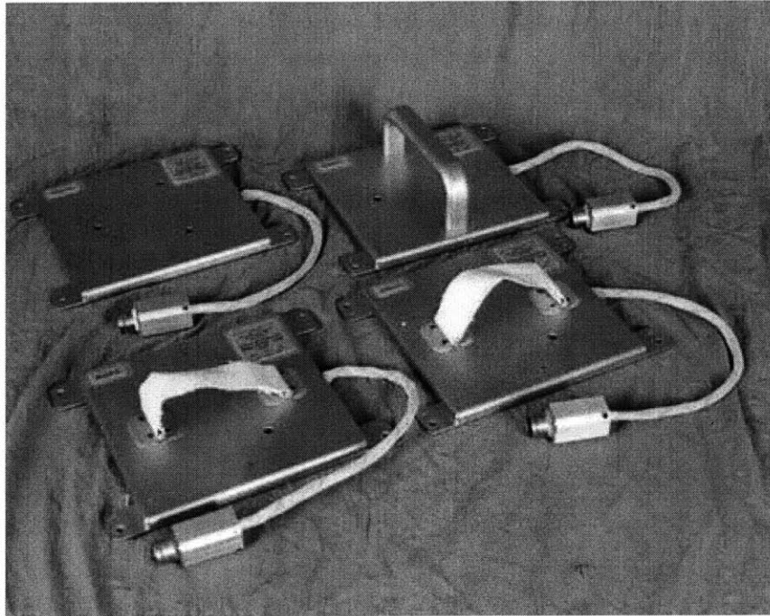
Figure B.1: This photograph shows four sensors as used for designing and testing the MICRO-G prototype. It includes a handhold, a touchpad and two foot restraints.
