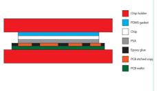
Chip bonding was achieved via the pressure sensitive adhesive (PSA) layer. Fluidic connections through a e (PDMS) made polydimethylsiloxane gasket to ensure leakage-free connections. The etched PCB was covered with epoxy glue. The glue was then ground until copper electrodes were revealed in order obtain a smooth, flat surface. Finally, pressure was maintained by screwing the whole system in a custom made chip holder.
