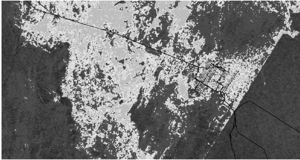
Fig. 5 Backscattering coefficient (dB) calculated from PALSAR L-band microwave data in Tokar region in Eastern Sudan: November, 2009). (Building and mesquite forest shows high dB; line: shows GPS tracking route)
