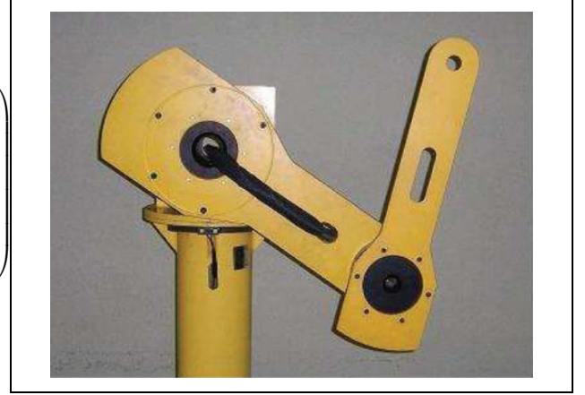
Figure 1. Experimental setup: two-DOF robot manipulator.
