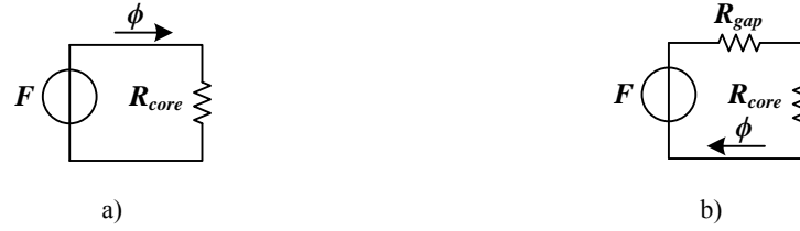
Fig 4.7. a) Equivalent magnetic circuit of the shell-type transformer. b) Equivalent magnetic circuit of the shell-type transformer with an air gap.
