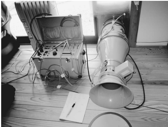
Figure 4. Measurement system of equivalent leakage area
