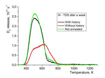
Fig. 4 TDS spectra of D<sub>2</sub> release from the annealed W sample with history, annealed and not annealed W samples without history, measured a week after the plasma exposure.
