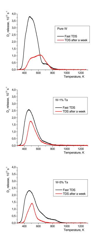
Fig. 2 Comparison of desorption spectra, recorded shortly after the first exposure of the sample with history ("fast TDS") and a week after the exposure (for the samples without history).
