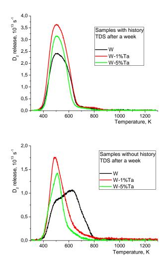
Fig. 1 TDS spectra of D<sub>2</sub> release from the samples of W, W-1%Ta and W-5%Ta with history and without history of previous exposures.
