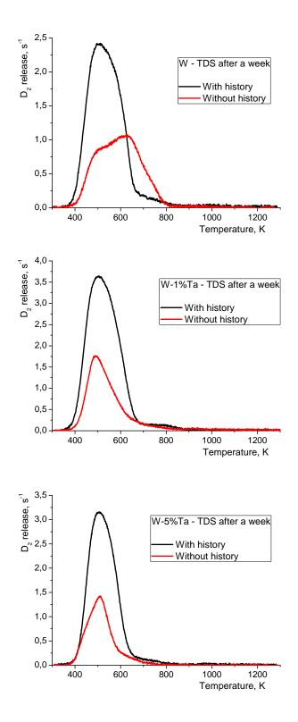
Fig. 3 Comparison of the spectra of D<sub>2</sub> release, recorded a week after the exposure, for the samples with and without history.
