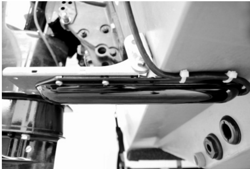
Figure 3.2 Mounting location of Skimmer® Imaging Transducer on vessel transom.
