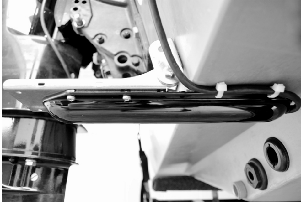
Figure 4.3 Mounting location of Skimmer® Imaging Transducer on vessel transom.
