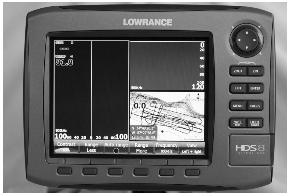
Figure 4.2 HDS-8 head unit showing side scan (left) down scan (upper-right) and charting (lower-right)
