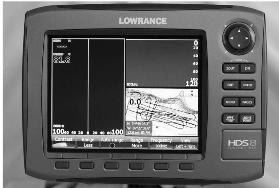
Figure 3.3 HDS-8 head unit showing side scan (left) down scan (upper-right) and charting (lower-right)
