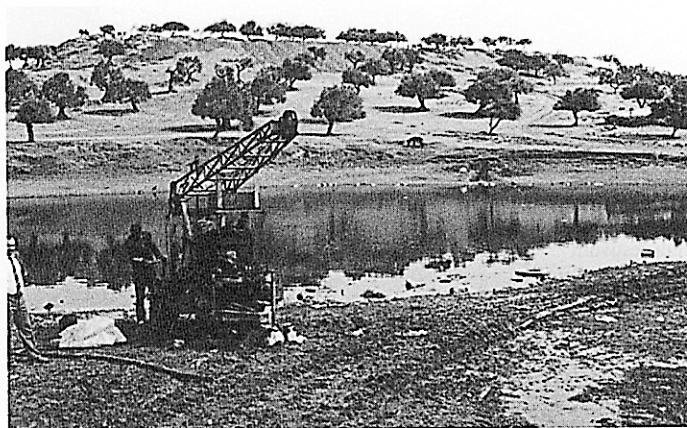
Fig. 6. Coring by the machine drill sampler in the pond. Behind hill is the Tell Mastuma.
