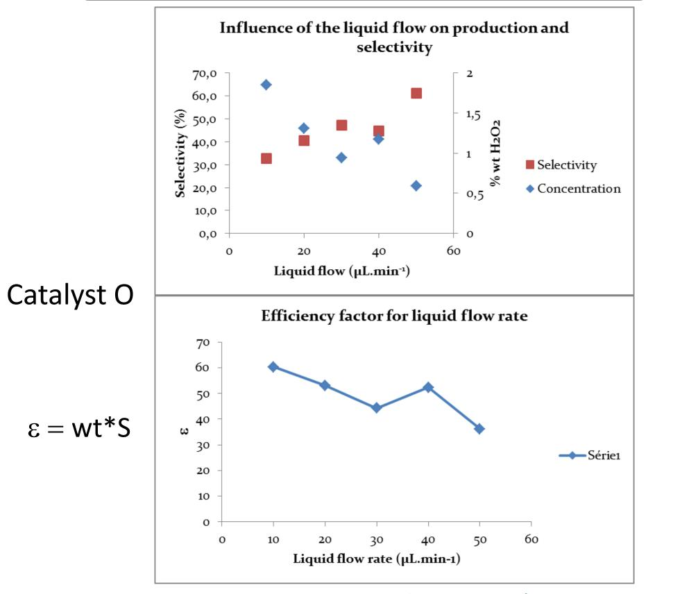
Increasing the total liquid flow rate (with a total gas flow of 1.25 mL.min<sup>-1</sup>) enabled us to reach a selectivity of 60%, but  $H_2O_2$  production remained low in these conditions. The efficiency factor  $\varepsilon$  suggests that we should work with higher liquid flow rate to obtain high selectivity. However to reach a satisfactory concentration ( $\geq 1\%$  wt  $H_2O_2$ ), we plan to work with moderate liquid flows.
