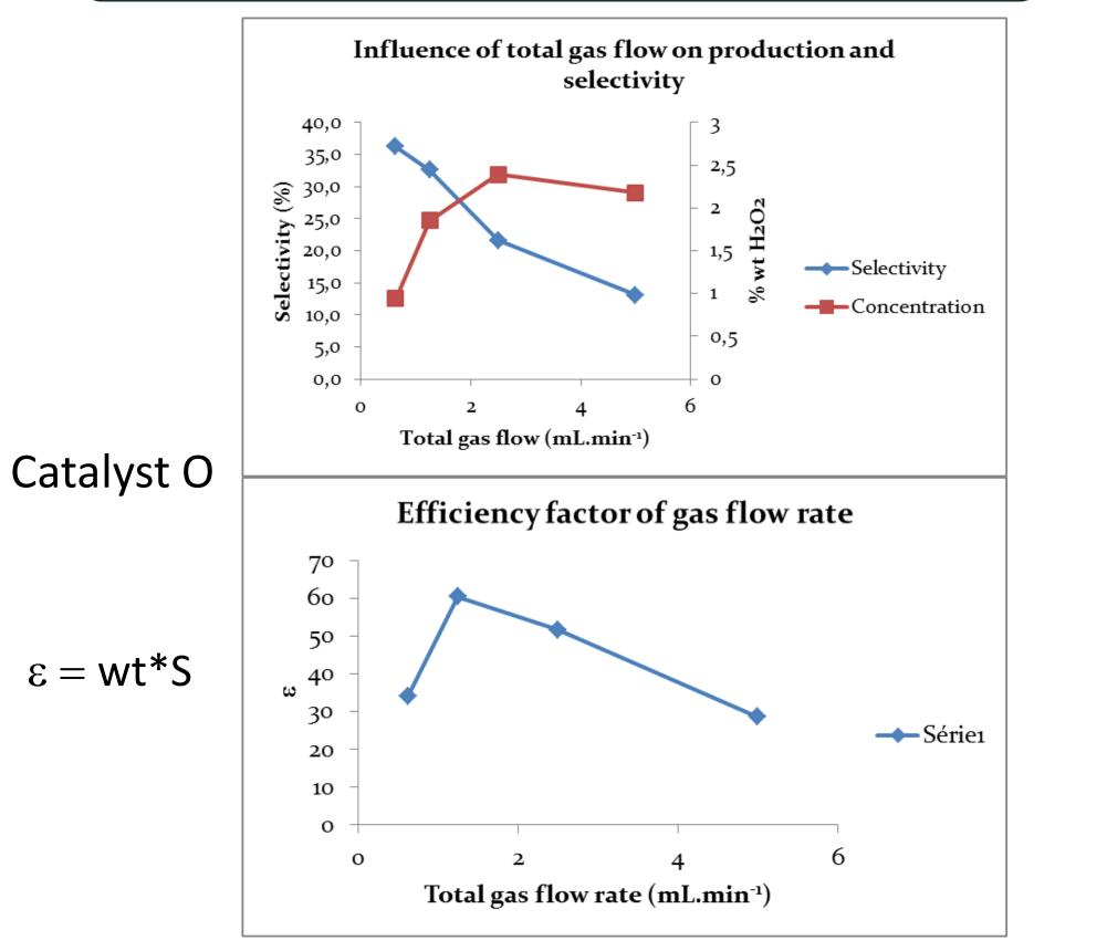
Increasing the total gas flow rate resulted in 2-fold improvement of  $H_2O_2$  production. However, the selectivity is decreasing with high gas flow rate. By looking at the efficiency factor  $\varepsilon$ , we concluded that working with a total gas flow rate of 1.25 mL.min<sup>-1</sup> seemed to be the best compromise between  $H_2O_2$ production and selectivity.
