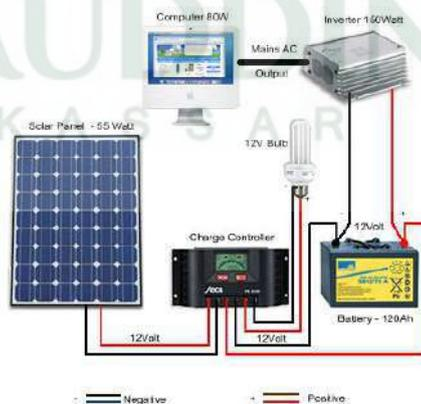
Gambar III.34. Sistem solar panel sederhana
