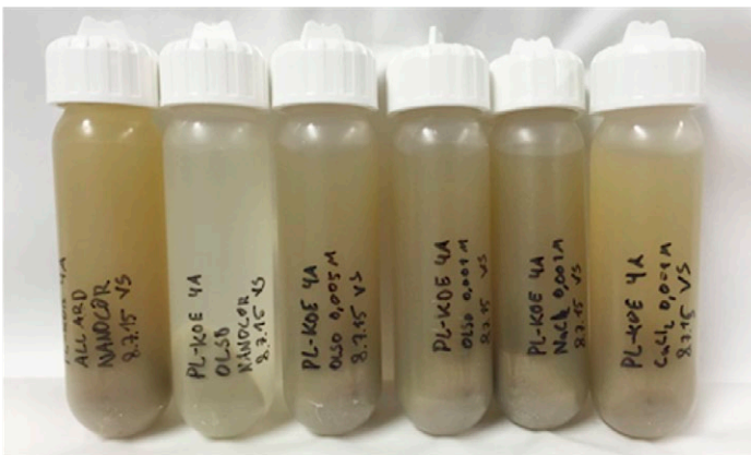
Figure 9. Nanocor PGN montmorillonite erosion experiment in different ionic strength reference ground water and electrolyte. From left: Allard (4.2 mM), Olso (0.52 M), Olso (5 mM), Olso (1 mM), NaCl (1 mM) and \text{CaCl}_2 (1 mM).
