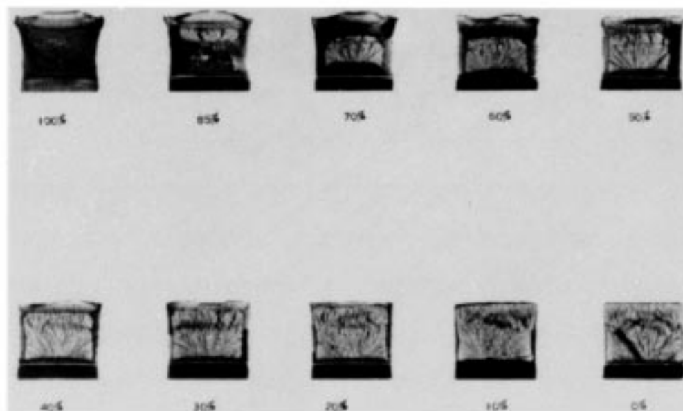
(a) Fracture Appearance Charts and Percent Shear Fracture Comparator
