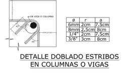
DETALLE DOBLADO ESTRIBOS EN COLUMNAS O VIGAS
