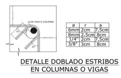
DETAILLE DOBLADO ESTRIBOS EN COLUMNAS O VIGAS
