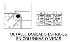
DETALLE DOBLADO ESTRIBOS EN COLUMNAS O VIGAS
