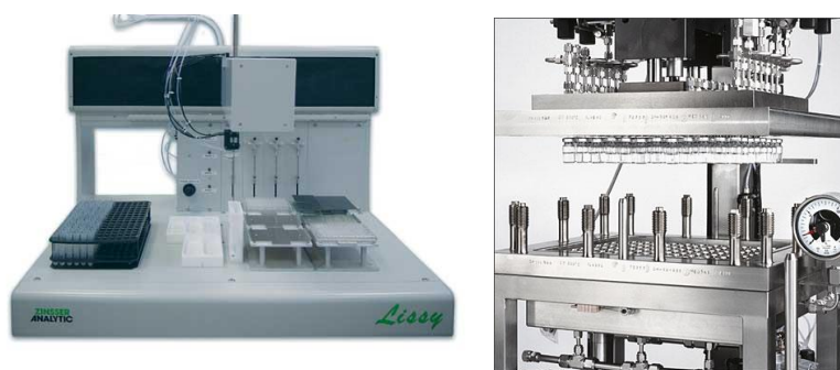
Figure S1: Hardware available at InnoSyn for high throughput screening: a) Liquid handling robot (Zinsser Lissy) and b) Premex 96-Multi Reactor. [1]
