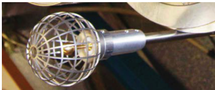
Figure 3.2: Positive ion probe as flown by the Technische Universität Graz. Same version was flown on WADIS-2 sounding rocket.
