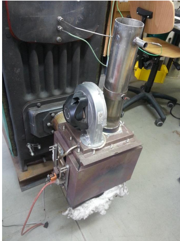
Figure 3-10. Open view of the Pyro-Man burner.
