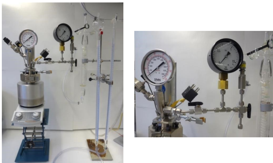
Figure 8: Modified autoclave setup. [118]
