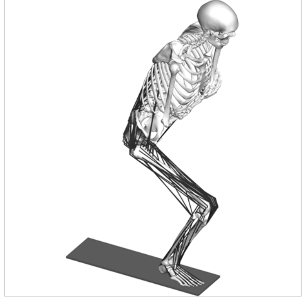
Fig. 3.3 Musculoskeletal model of the lower right extremity with the upper body attached as one rigid segment and an implanted THR.
