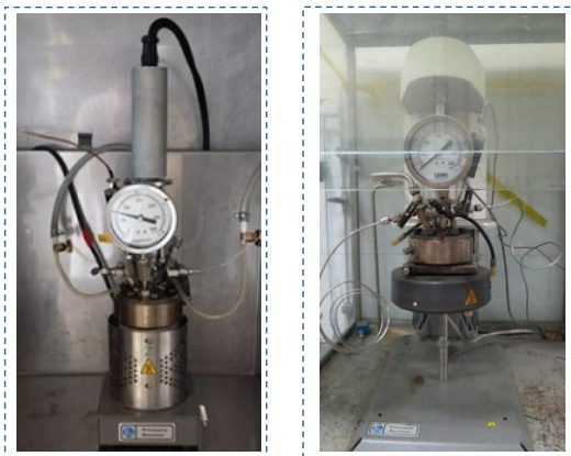
Figure A1. Experimental set up (autoclave) of HDO of phenol (left) and bio-oil (right).
