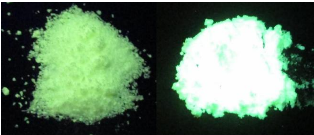
Figure 3.8.5.5. [\text{Tb}(\text{H}_2\text{O})_7][\text{B}(\text{CN})_4]_3 (left) and dried [\text{Tb}(\text{H}_2\text{O})_n][\text{B}(\text{CN})_4]_3 ( n = 1-0 ) (right) under ultraviolet light, with excitation wavelength, \lambda = 254 nm.
