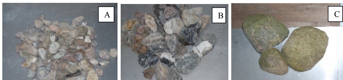
Figure 3.3 River stone medium: A (16-32mm); B (32-64mm) and C (80-100mm, Support)
