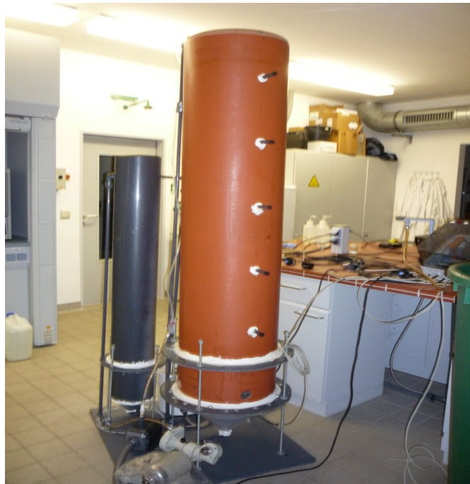
Figure 3.2 The pilot scale trickling filter
