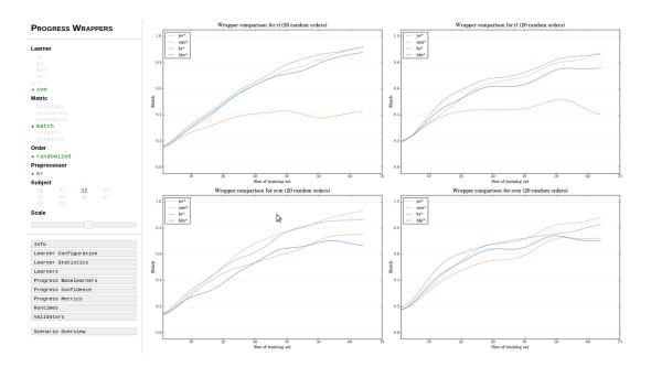
Figure 6.20: Screenshot of DILES plot compositions. This example shows plots which compare the progress of different performance metrics (during the iterative evaluation process) for the used wrapper methods. If the mouse pointer is moved over a specific plot, the corresponding parameters in the sidebar are highlighted.
