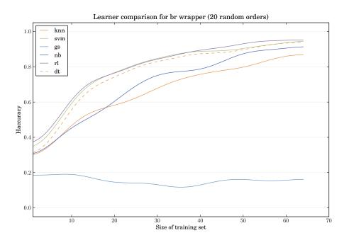
**Figure 6.11:** Example plot of DILES' evaluation result analysis. Progress of the metric *h*-accuracy for all base learners in combination with a Binary Relevance (BR) wrapper.
