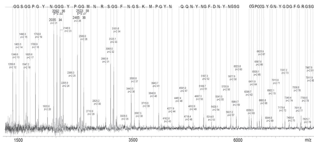
**Figure 3:** MALDI ToF ISD spectrum of HPLC purified recombinant RA33. Fragment ion signals are recorded in the mass range of  $m/z$  1000 to 8000. The ion signals cover the C-terminal sequence from aa 234 to aa 305. In the sequence gaps occurred at residues Asn253-Tyr254 at Pro269-Ser270, and at Gly298-Gly299-Ser300, respectively. Z+2 ions are labeled. Matrix: DHB.
