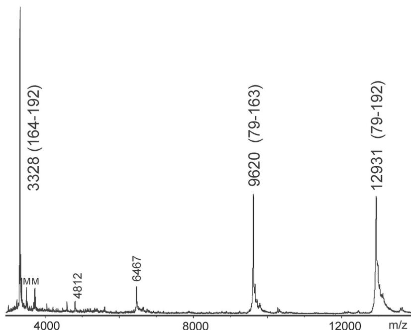
**Figure 7:** MALDI ToF MS analysis of a protein fragment from immuno-positive HPLC fraction 8 (*cf.* Figure 6). The spectrum was recorded in linear mode ( $m/z$ : 3000–35,000). The region from  $m/z$  3000–14000 is shown. Peptide ion signals are labelled with  $m/z$  values. Matching amino acid sequence ranges are shown in parentheses. For complete assignments *cf.* Table 3. M indicates matrix adducts. Matrix: DHB.
