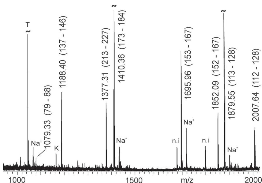
**Figure 5:** MALDI ToF MS peptide mapping analysis after *in-gel* trypsin digest of BrCN-derived protein fragments from immuno-positive band 8 of the SDS PAGE analysis (*cf.* Fig. 4). Peptide ion signals are labeled with  $m/z$  values. Matching amino acid sequence ranges are shown in parentheses. T indicates ion signals due to trypsin auto-proteolysis. Matrix: CHCA.
