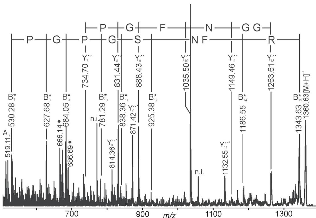
**Figure 3:** MALDI-QIT-ToF MS/MS spectrum of the ion signal at  $m/z$  1377.63 (*cf.* Fig. 2). The determined partial amino acid sequence is depicted and was assigned to an RA33 peptide comprising amino acids 213-227. The mass spectrometric fragment ions from the Y"-type ion series and the B-NH<sub>3</sub>-type ion series are indicated. The asterisk indicates loss of ammonia. A dot symbol indicates an internal fragment. DHB was used as matrix.
