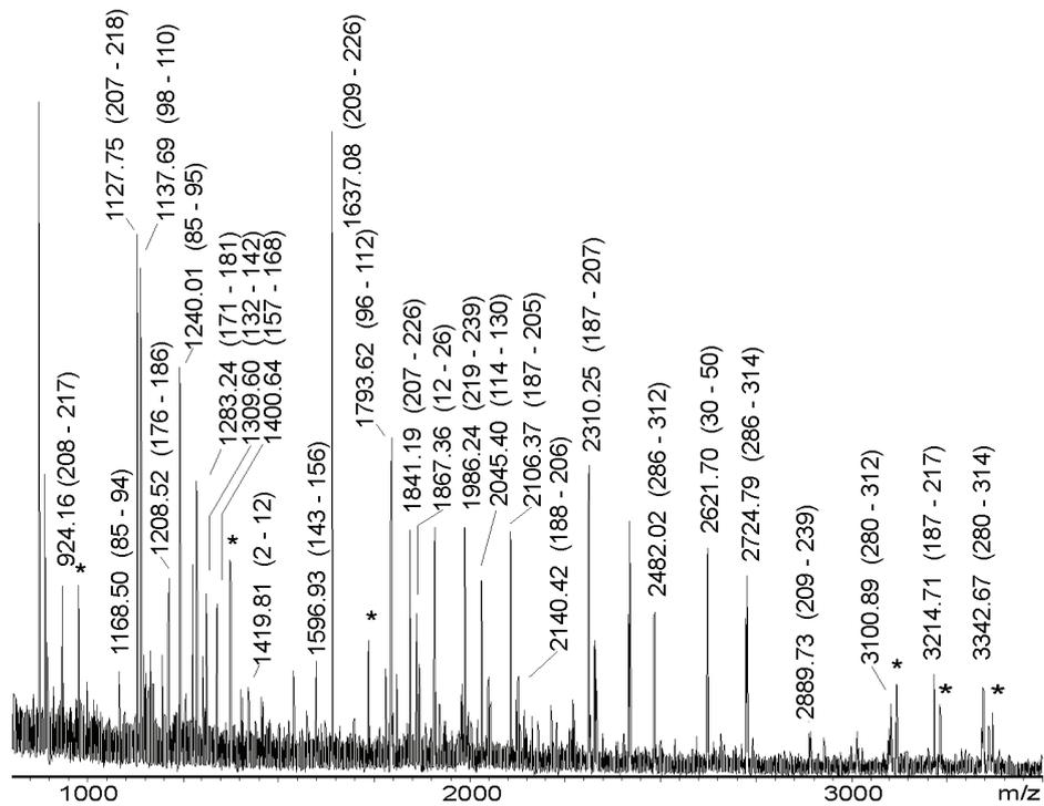
**Supplemental Figure 3:** MALDI ToF MS analysis of thermolytic digest of RA33. Peptide ion signals are labeled with *m/z* values. Matching amino acid sequence ranges are shown in parentheses. The asterisk indicates oxidation. Matrix: DHB.
