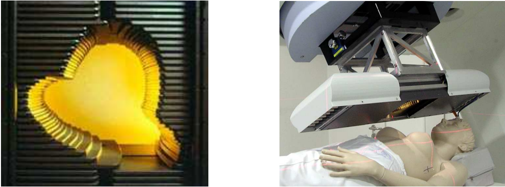
Fig. 1.1: Multileaf collimator and linear accelerator. Left: The leaf pairs of a multileaf collimator that can be shifted to form differently field shapes. Right: The linear accelerator and the treatment couch with gantry and beam head.
