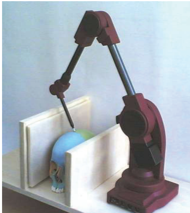
Abbildung 36: MicroScribe® G2 3D Digitizer von Immersion Corporation (US)
