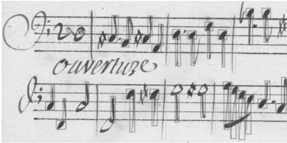
Figure 3.3: A Region of Interest (ROI) from a music manuscript image and MBRs of the detected music objects
